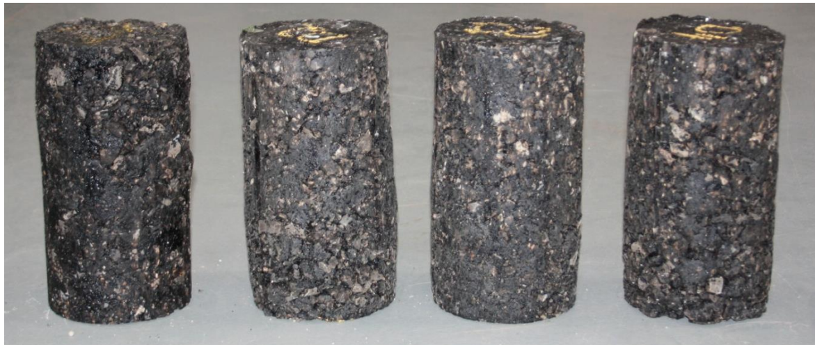
Figure 6: Typical examples of failed test specimens
