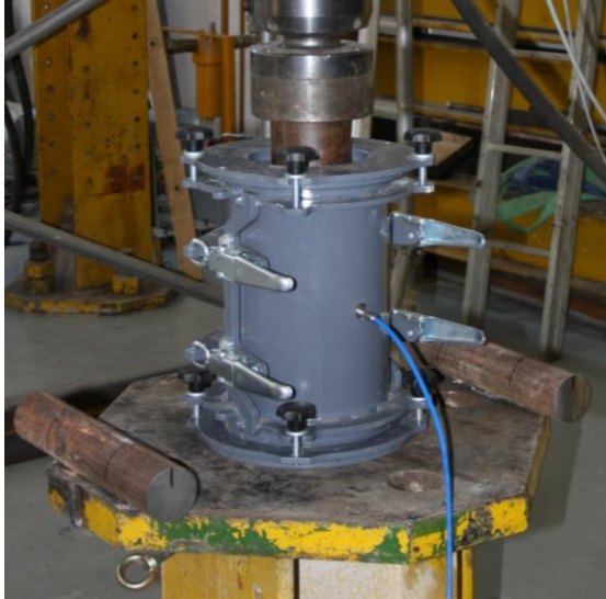
Figure 4: Stressing the test specimens during the tests
