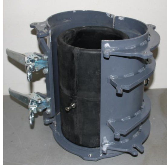
Figure 5: Detail of the special mould with rubber membrane inside
