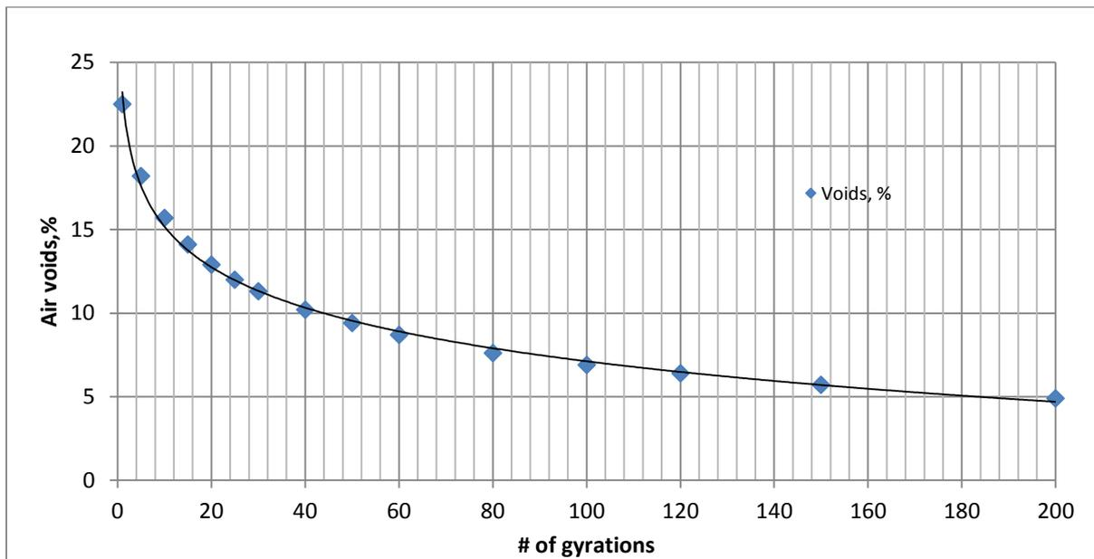
Figure 2: Example of a densification curve of the BBSG 0/10 Class 3
