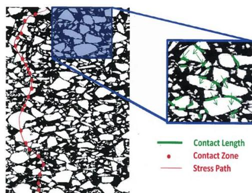
Figure 4. Digital Image and method of determining the contact length [7].
