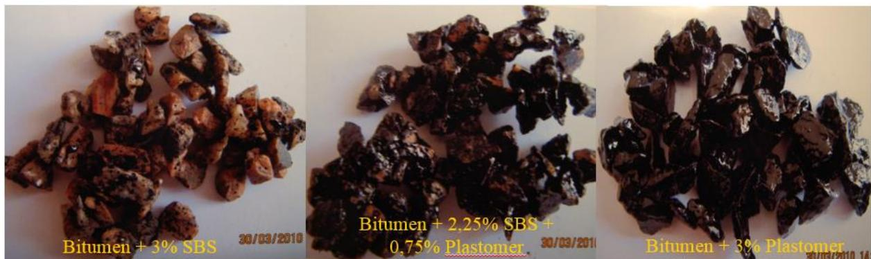
Figure 3: Boiling water test results (left = pure SBS, middle = hybrid, right = pure plastomer)
