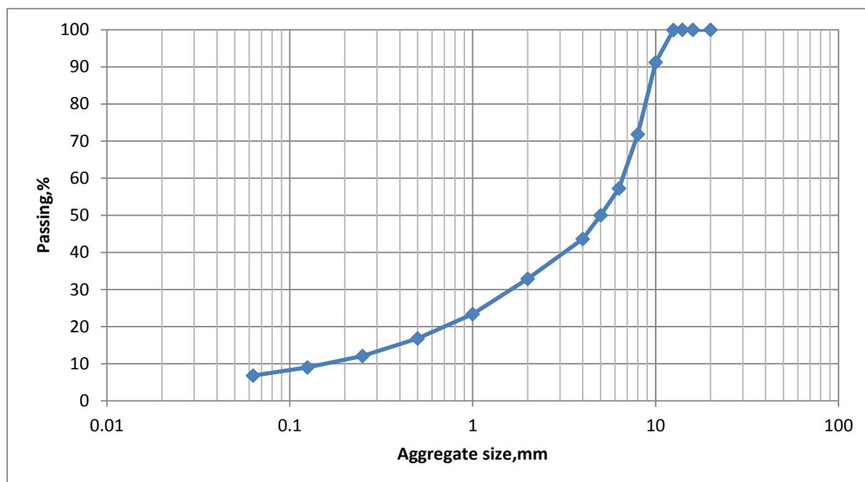
Figure 1: Gradation curve of the BBSG 0/10 Class 3
