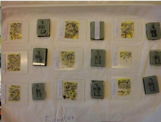
f) Thin sections for microscope test
