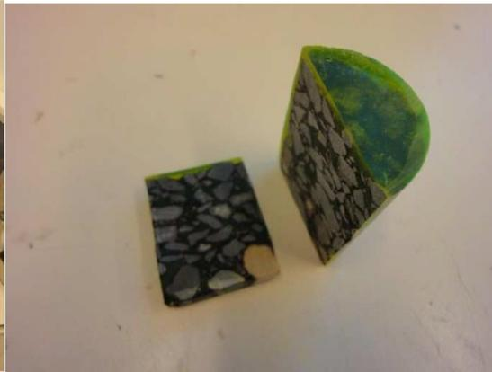
b) The sample saturated with epoxy resin
