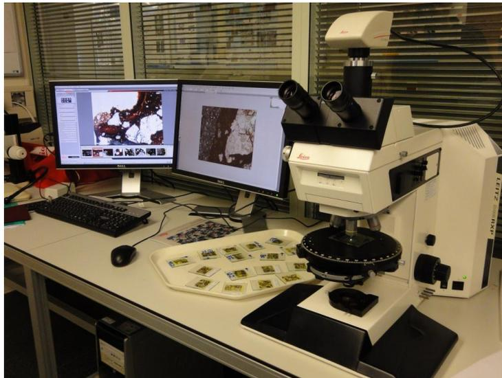
Figure A3. Picture of the Polarizing Microscope (LEITZ DM RXP) in the Microlab of TUDelft
