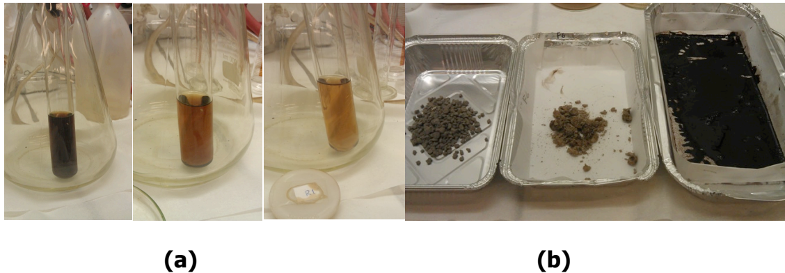
Figure 5. (a) From left to right are the dichloromethane after 1 st , 4 th and 7 th centrifuge rotation. (b) From left to right are the granular RETONA in original form, the filler, and the bitumen extracted.
