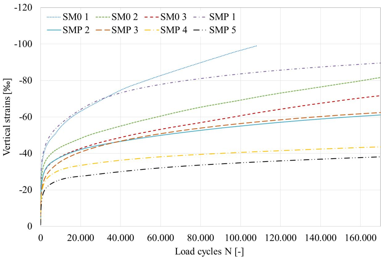
**Figure 7: Vertical plastic strains of the eight asphalt surface course variations during UCCT**
