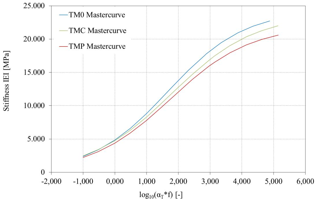
**Figure 5: Mastercurves and single stiffness values of the three asphalt base variations**
