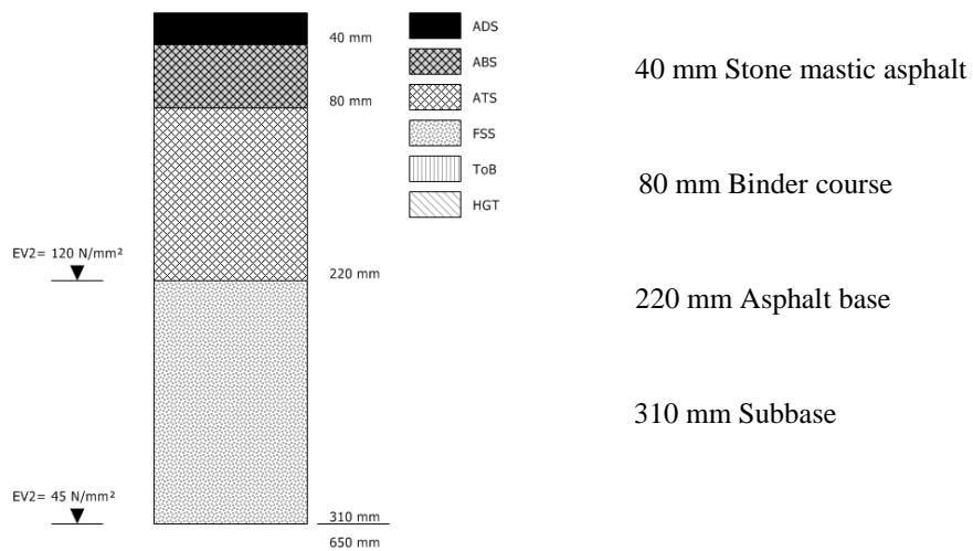
**Figure 8: Layer structure of the chosen pavement**
