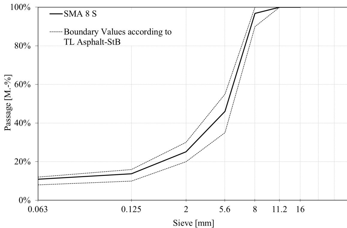
**Figure 2: Grading chart for the eight asphalt surface course variations SMA 8 S**
