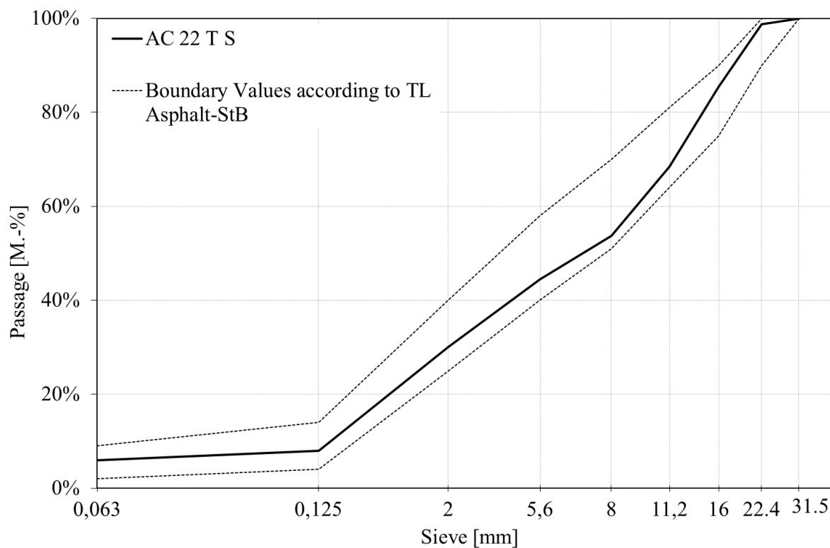
**Figure 1: Grading chart for the three asphalt base variations AC 22 T S**
