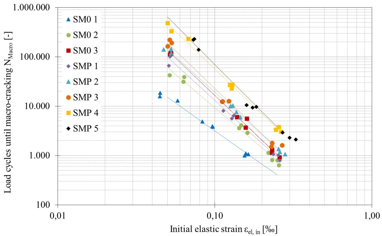
**Figure 4: Fatigue characteristics of the eight asphalt surface course variations**
