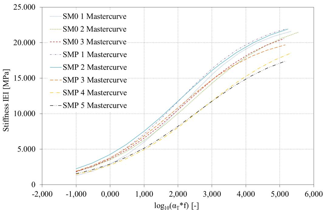
**Figure 6: Mastercurves of the eight asphalt surface course variations**
