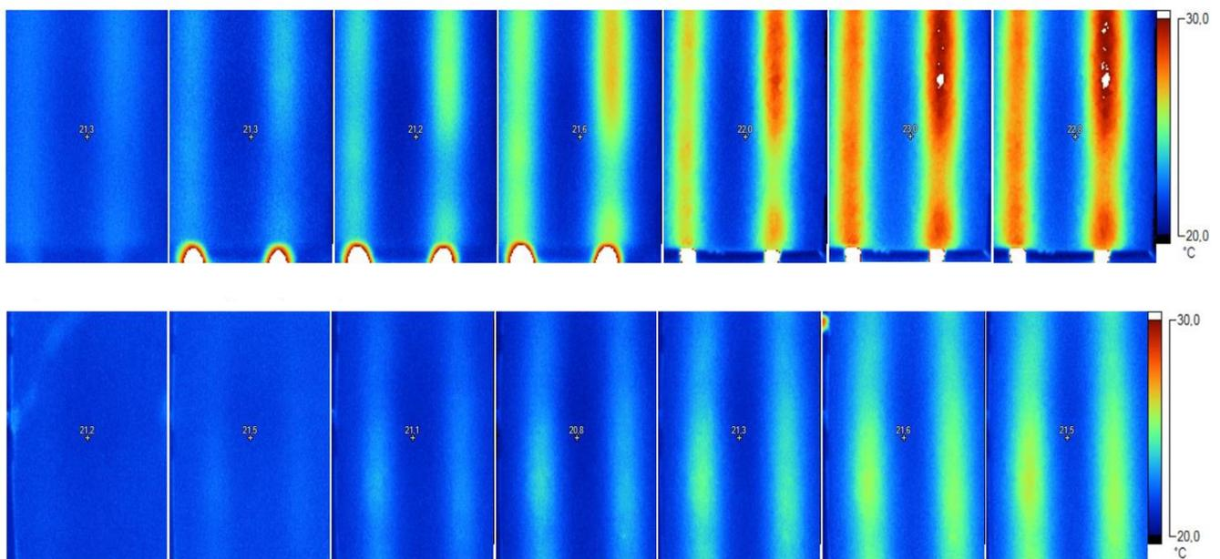
**Figure 9: Heating up of the asphalt surface with 50 W/m<sup>2</sup>, the two ribbons on the right of the slab (with insulation) at a depth of 4 (upper row) and 8 cm (lower row) respectively**
