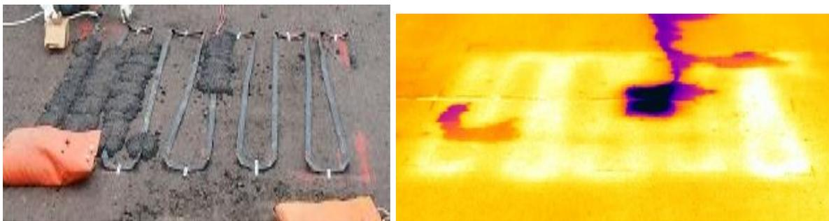
**Figure 16: Infra-red photo of the 10 cm depth heated area**
