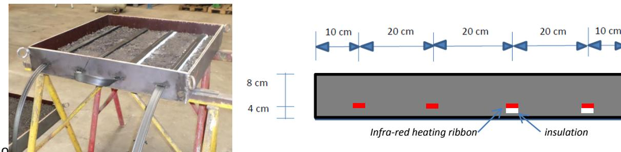
**Figure 7: Infra-red heating ribbons built in asphalt trial, 8 cm under surface, partly with insulation (under two right ribbons)**
