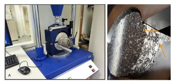
Figure 2: Shear bond strength test equipment and specimen.
