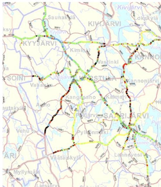
Figure 7. Annual rut growths (100m average) and annual paving costs in the Karstula maintenance area in Central Finland.
