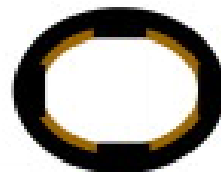
Virgin large aggregate + RAP binder + virgin binder
