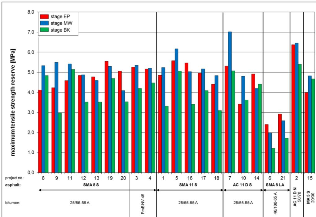
Figure 8: Maximum tensile strength reserve of the 21 sections
