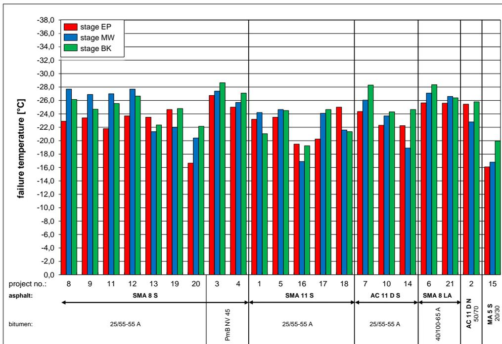
Figure 4: Failure temperatures of the 21 sections at the three stages
