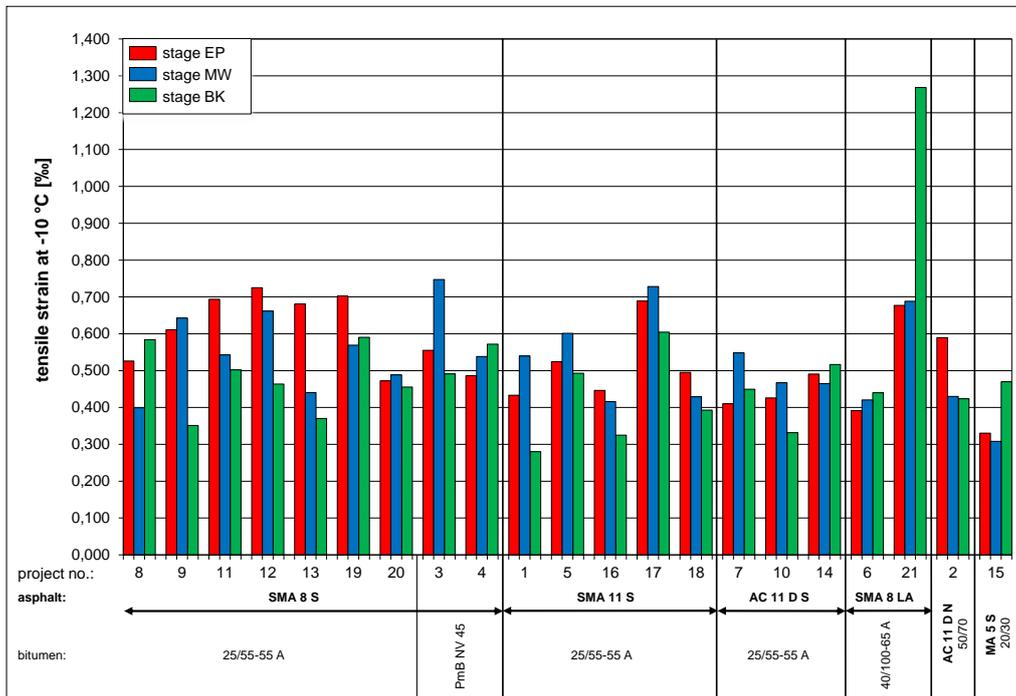
Figure 7: Tensile strain at -10 °C of the 21 sections at the three stages
