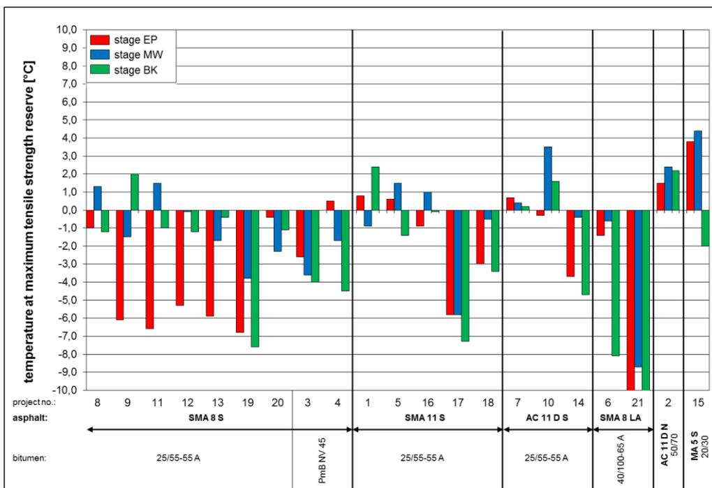
Figure 9: Temperature associated to the maximum tensile strength reserve of the 21 sections
