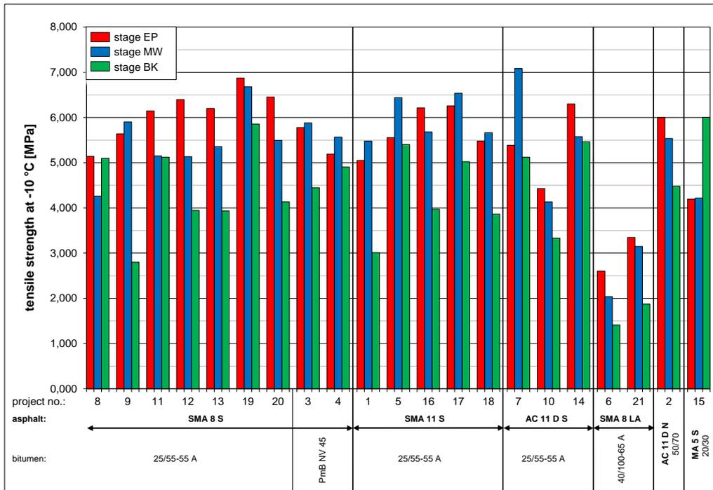
Figure 6: Tensile strength at -10 °C of the 21 sections at the three stages
