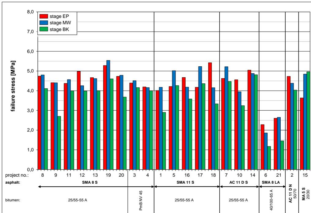
**Figure 5: Failure stress of the 21 sections at the three stages**
