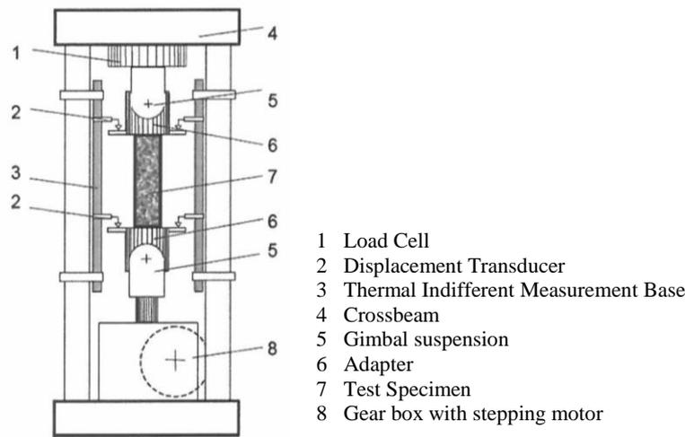
**Figure 2: Test set-up to perform TSRST and UTST**
