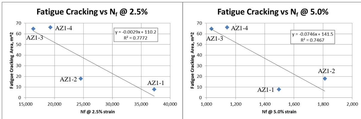
Figure 8. Field fatigue cracking data vs. LAS test  $N_f$  values at (a) 2.5% strain and (b) 5.0% strain.
