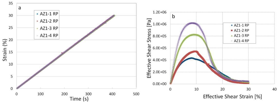
**Figure 3 (a): recorded strain, and (b): apparent stress response from the continuous strain sweep.**
