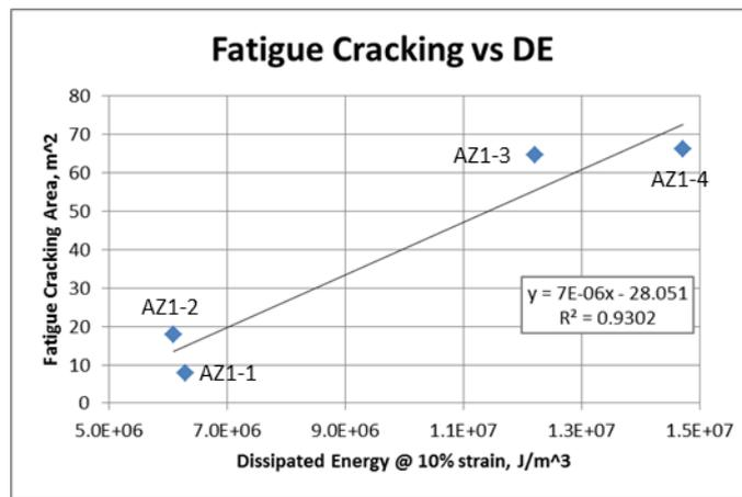
Figure 9. LAOS test dissipated energy (DE) values vs. field fatigue cracking data.
