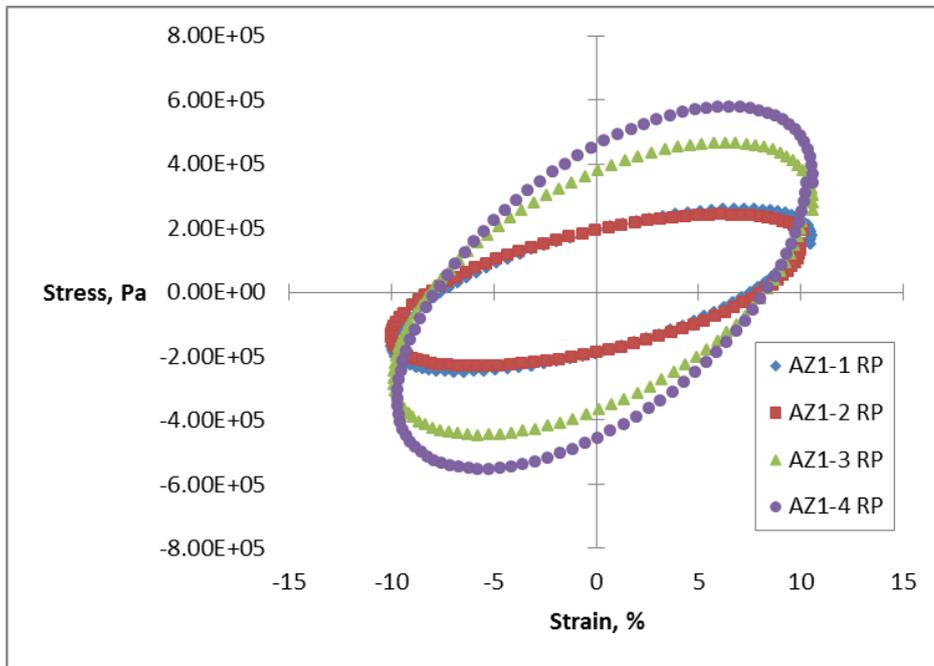
Figure 6. Lissajous curves for each sample at 28C and 10% strain.
