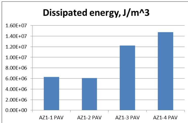
Figure 7. Calculated dissipated energies for samples AZ1-1,2,3, and 4.
