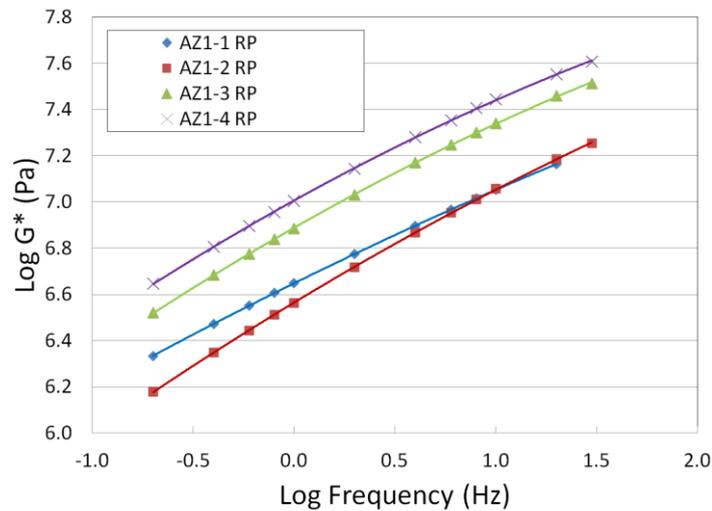
Figure 2. AZ bitumens: frequency sweeps at the intermediate test temperature (28°C).
