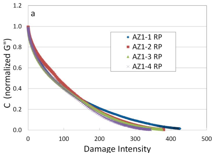
**Figure 4. AZ1-1, 2, 3, and 4. Normalized loss modulus,  $G''$  versus damage from LAS testing.**
