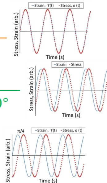
Figure 1. Linear viscoelasticity (small amplitude oscillatory shear (SAOS)).
