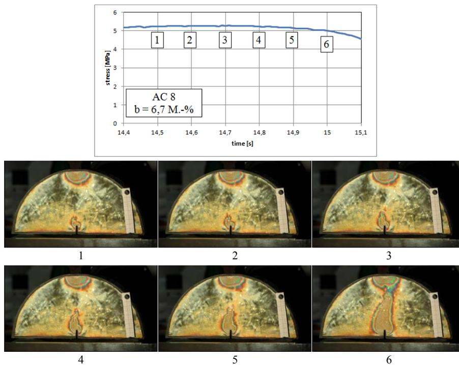
**Figure 8: Crack propagation in a monotonic bending test (AC 8)**
