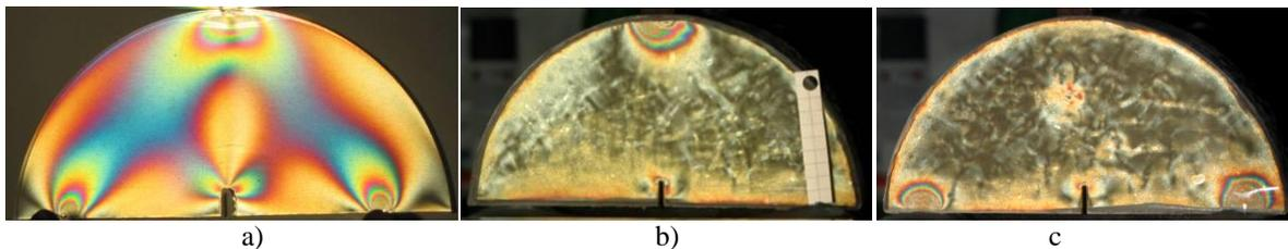
**Figure 6: a) Visualized isochromatics in a homogeneous and elastic specimen and b) and c) nearly no isochromatics on an asphalt specimen AC 8 under load.**
