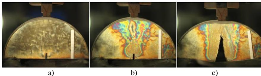
**Figure 11: Isochromatic patterns in a cyclic semi-circular bending test, after 258 load cycles (a), after 12,900 load cycles (b) and after 13,100 load cycles (c)**
