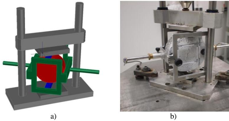
**Figure 5: a) Sketch for Cyclic Indirect Tensile Test and b) experimental setup with specimen**
