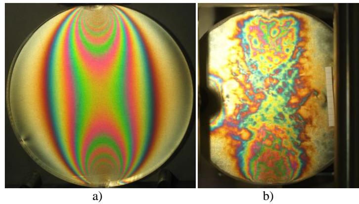
**Figure 13: a) Visualized isochromatics in a homogeneous and elastic specimen and b) isochromatics on an asphalt specimen AC 8 after 300 load cycles.**
