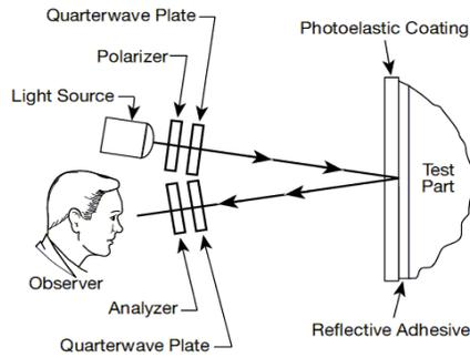
**Figure 3: Principle of the reflection polariscope [8, 9, 10]**
