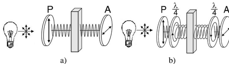
**Figure 1: Principles of photoelasticity a) plane polarized light, b) circular polarized light**
