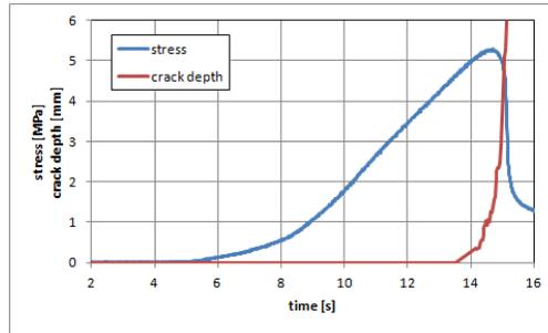
**Figure 9: Crack growth for asphalt mixture AC 8**
