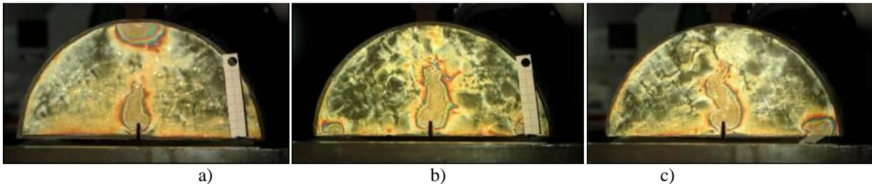
**Figure 10: Crack line for asphalt mixtures a) AC 8, b) AC 16 and c) AC 22**
