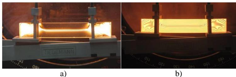
**Figure 2: View on a sample rayed by monochromatic a) plane polarized light and b) circular polarized light.**
