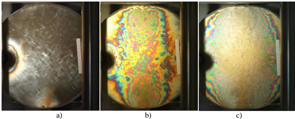
**Figure 14: Isochromatic patterns in a cyclic indirect tensile test, at start (a), after 600 load cycles (b) and after 4,700 load cycles (failure) (c)**
