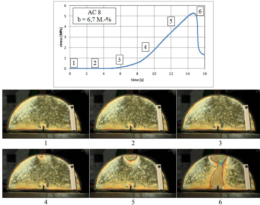
**Figure 7 Visualization of the deformation evolution during a monotonic bending test (AC 8)**
