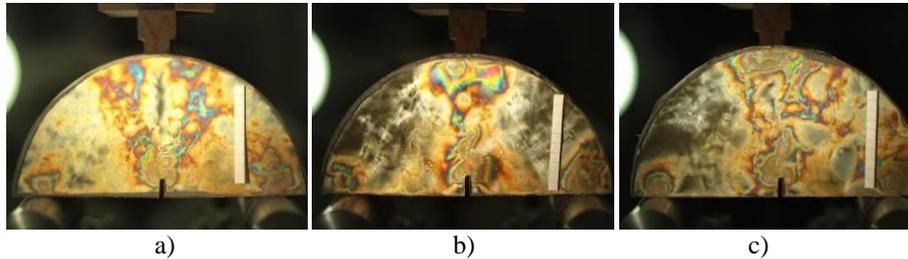
**Figure 12: Isochromatic patterns in a cyclic semi-circular bending test at ~90 % of the test duration. AC 8 (a), AC 16 (b) and AC 22 (c)**
