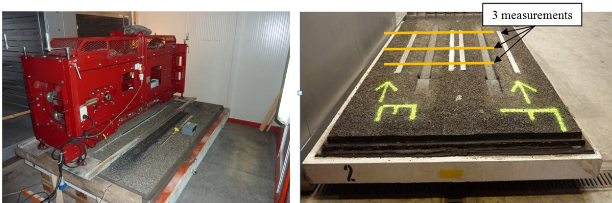
Figure 2: Left: Model Mobile Load Simulator MMLS3, right: 2 rutting profiles on system 5
