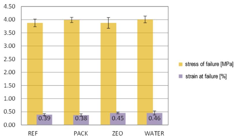
**Figure 9: Uniaxial Tension UTST at + 5 °C (EN 12697-46)**
