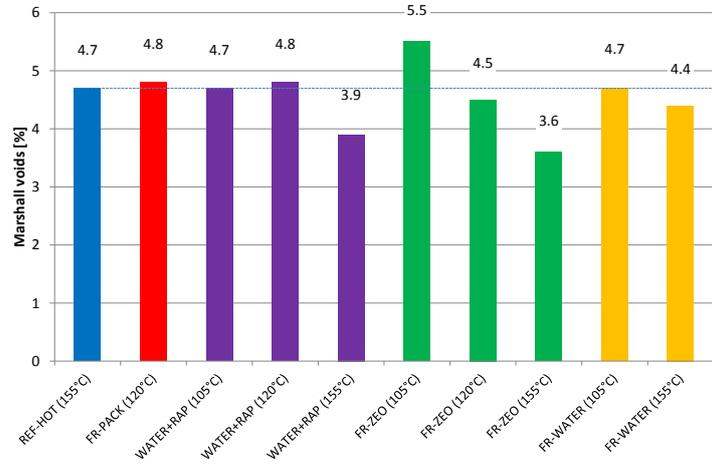
**Figure 2: Marshall (50/50 blows) voids for different reheating temperatures in the laboratory**
