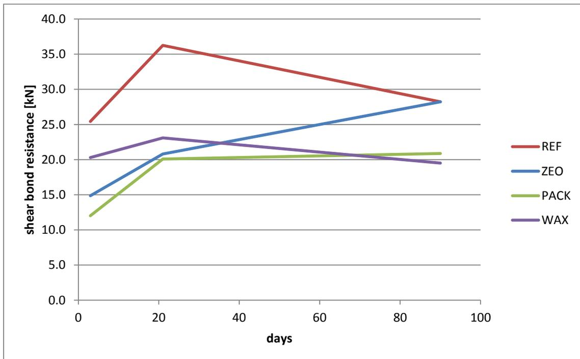
**Figure 6: Development of the layer-bonding under laboratory conditions**
