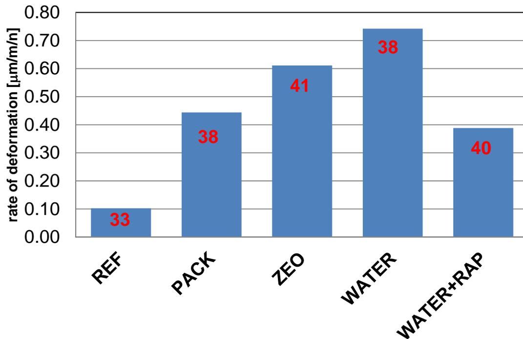
Figure 8: Triaxial compression test (EN 12697-25); Penetration of the binder in red
