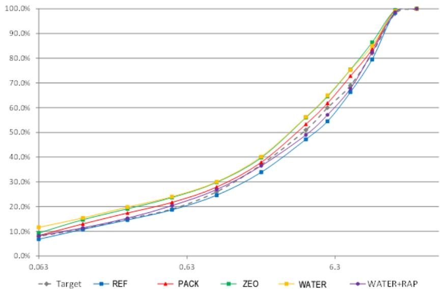
**Figure 3: Grading curve of the various mixtures tested**
