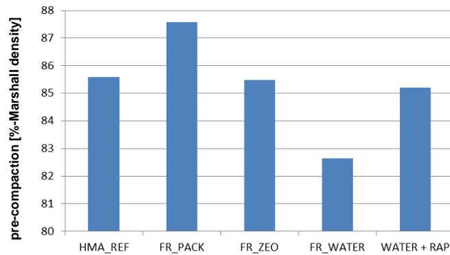
**Figure 1: Compaction directly behind the finisher**
