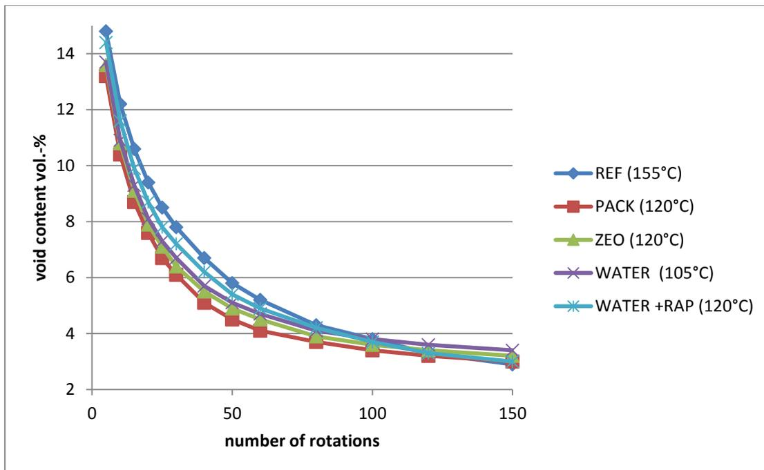
**Figure 4: void content as a function of the number of rotations in the gyratory-test**
