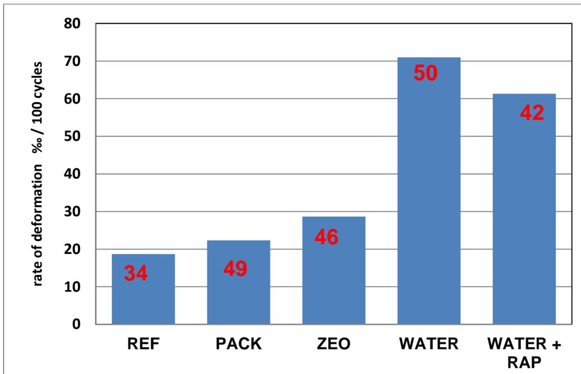
Figure 7: Uniaxial compression test (EN 12697-25); Penetration of the binder in red
