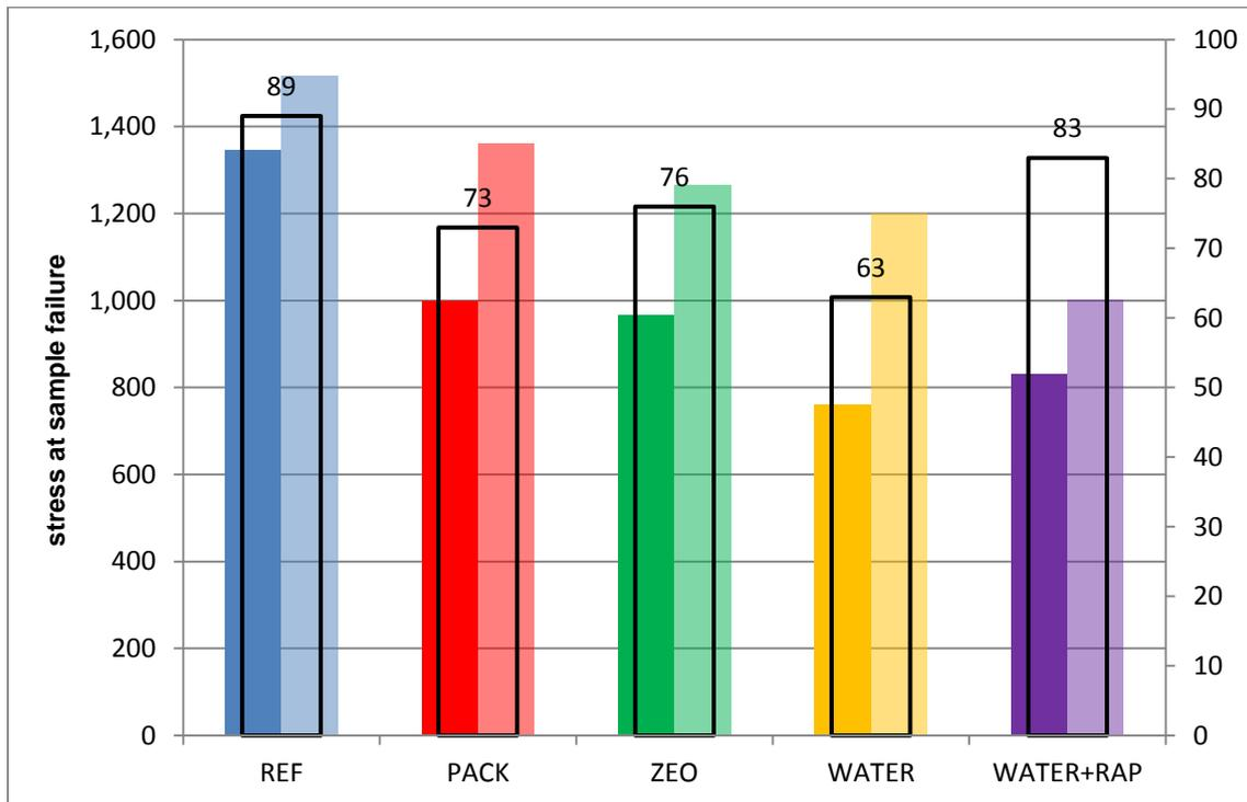
Figure 5: Water sensitivity tests according to EN 12697-12 (transparent colours for  $ITS_d$ / solid colours for  $ITS_w$  and black lines for ITSR ratio)
