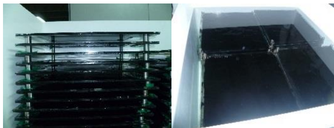
Figure 1: Arrangement of the asphalt submerged in aquaria (a); 2mm laminae on glass with lamina arrangement (b); submerged laminae
