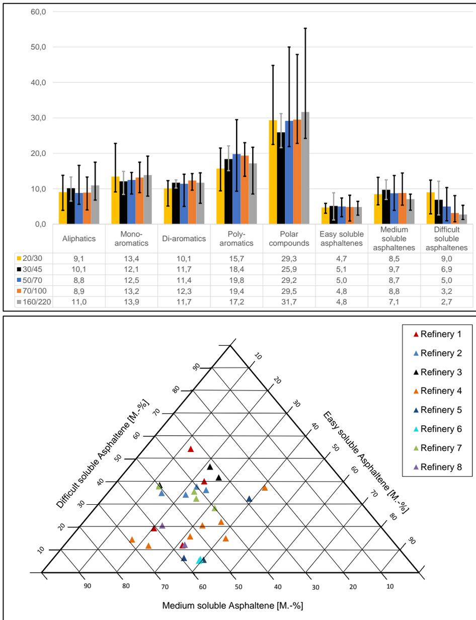
**Figure 4: SARA-analysis and separation into easy, medium and difficult soluble asphaltenes; for every bitumen grade the average value as well as the minimum and the maximum (top); ternary plot for easy, medium and difficult soluble asphaltenes of bitumens 50/70 form different refineries (down)**
