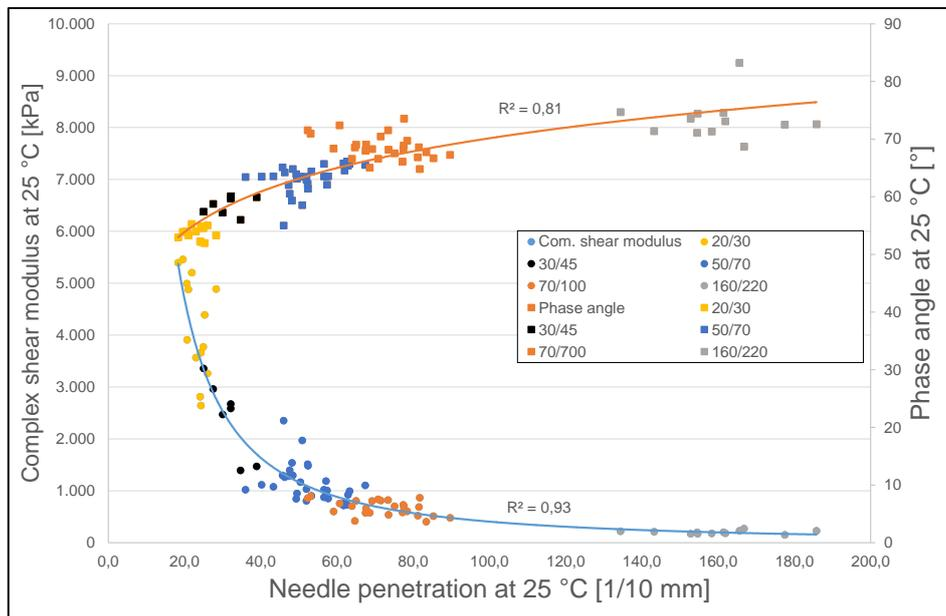
**Figure 8: Correlation between needle penetration and complex shear modulus resp. phase angle (each at 25 °C)**
