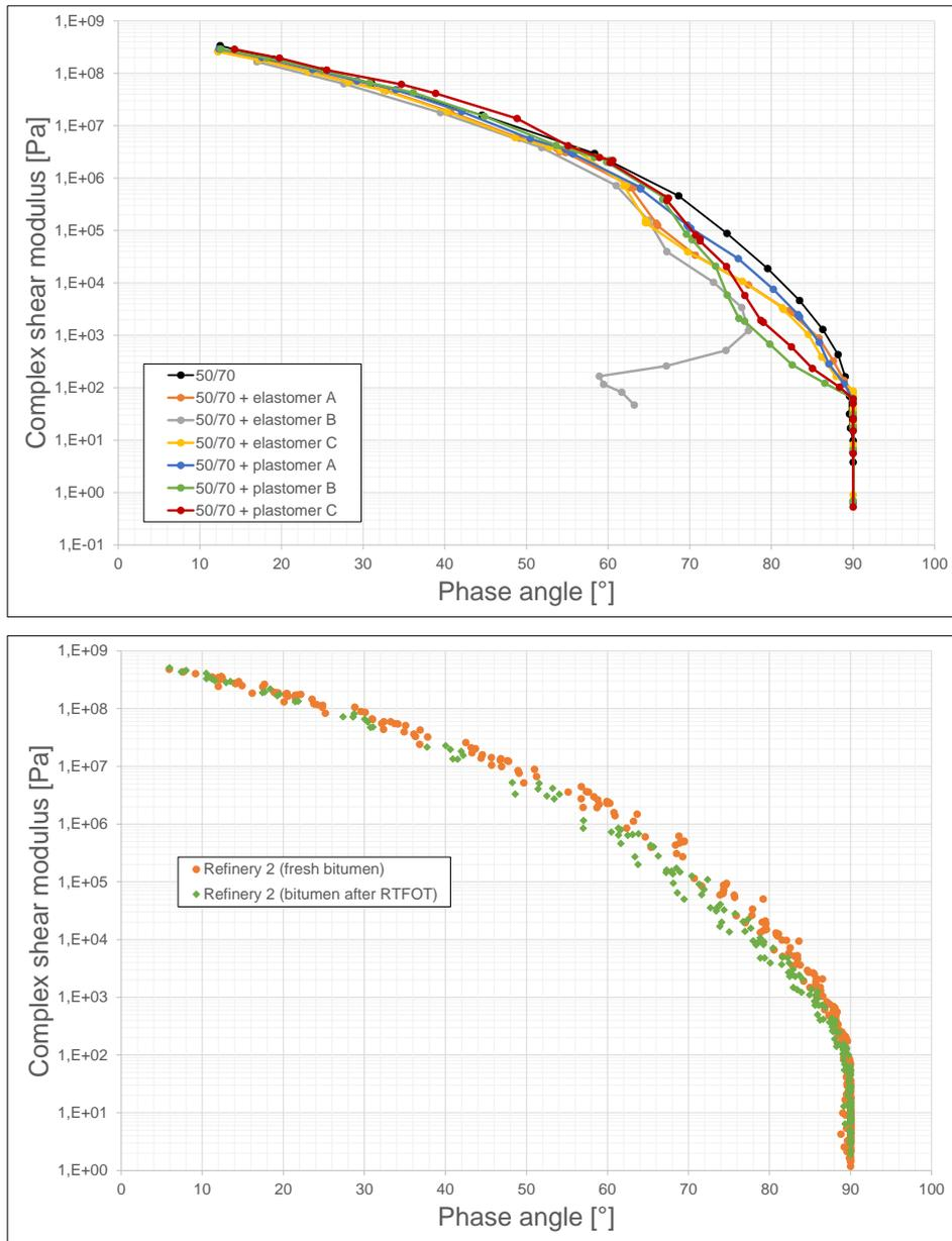
**Figure 11: top: Black-diagram of a bitumen 50/70 before resp. after modification with different polymers; down: Black-diagram of identical bitumens before and after short time aging (RTFOT)**
