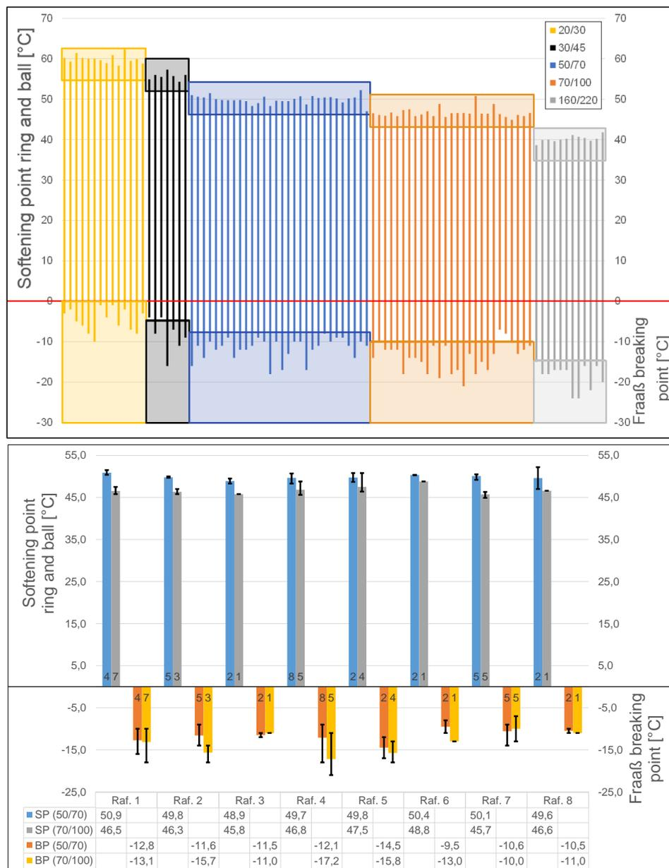
**Figure 2: Softening point ring and ball resp. Fraaß breaking point; top: all analyzed paving grad bitumens; down: average values and spread of bitumens 50/70 and 70/100, each depending on the refinery**
