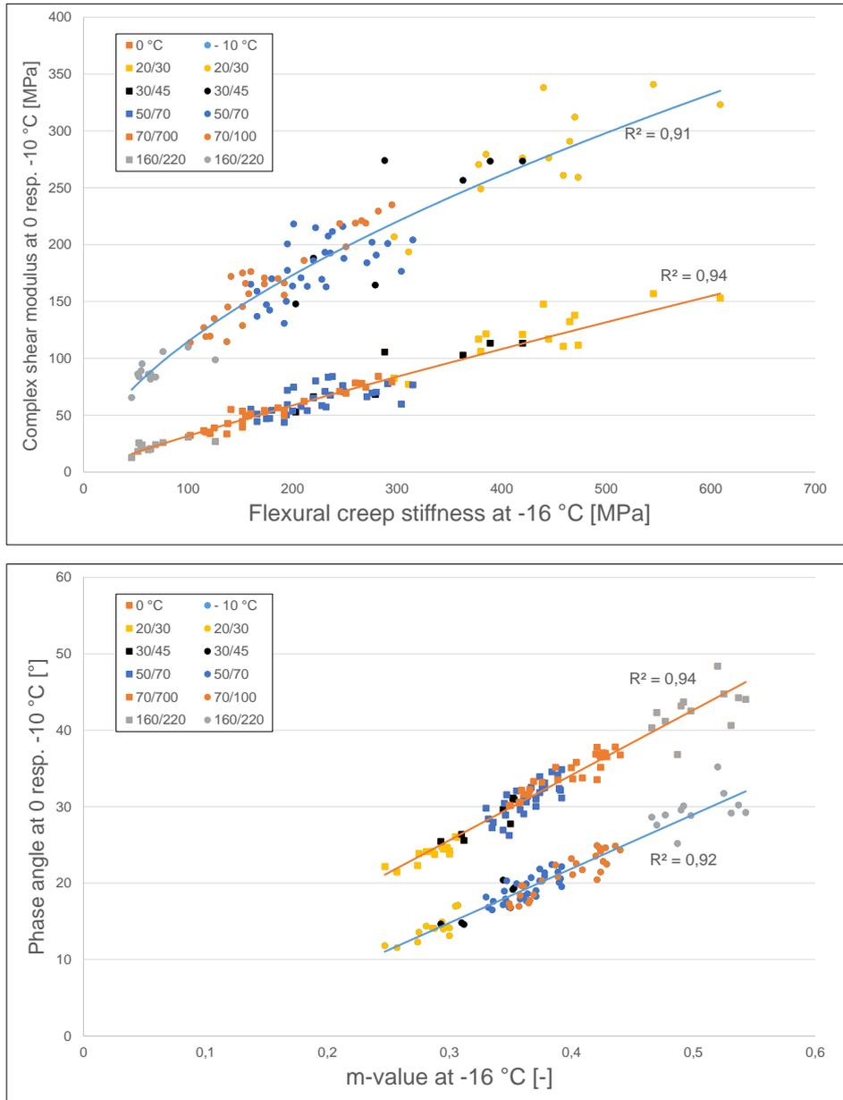
**Figure 7: Correlation between BBR results at -16 °C and DSR results at 0 resp. -10 °C; top: flexural creep stiffness of complex shear modulus; down: m-value of phase angle**
