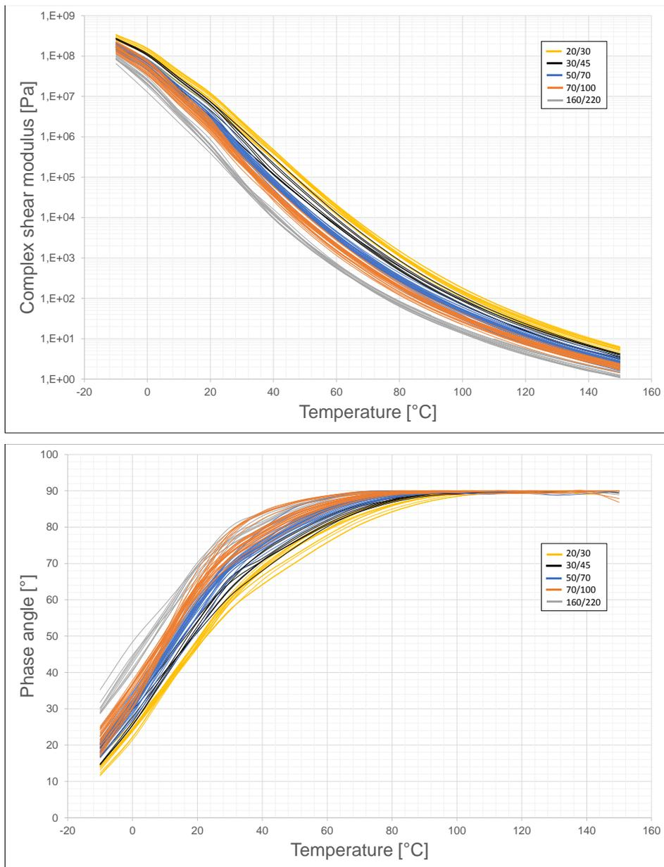
**Figure 3: Temperature dependent complex shear modulus (top) and phase angles (down) of the analyzed paving grade bitumens**
