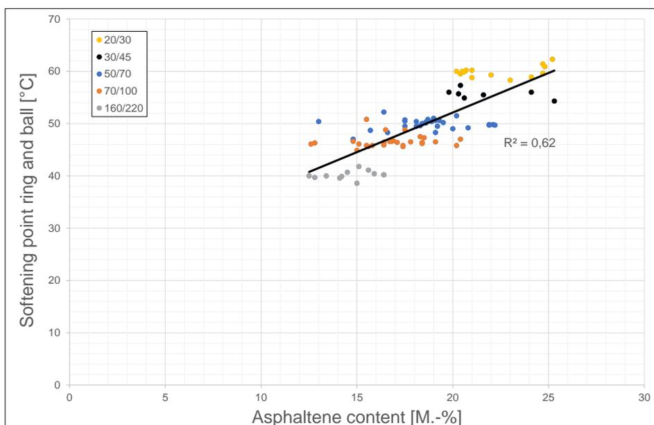
**Figure 6: Correlation between asphaltene content and softening point ring and ball**
