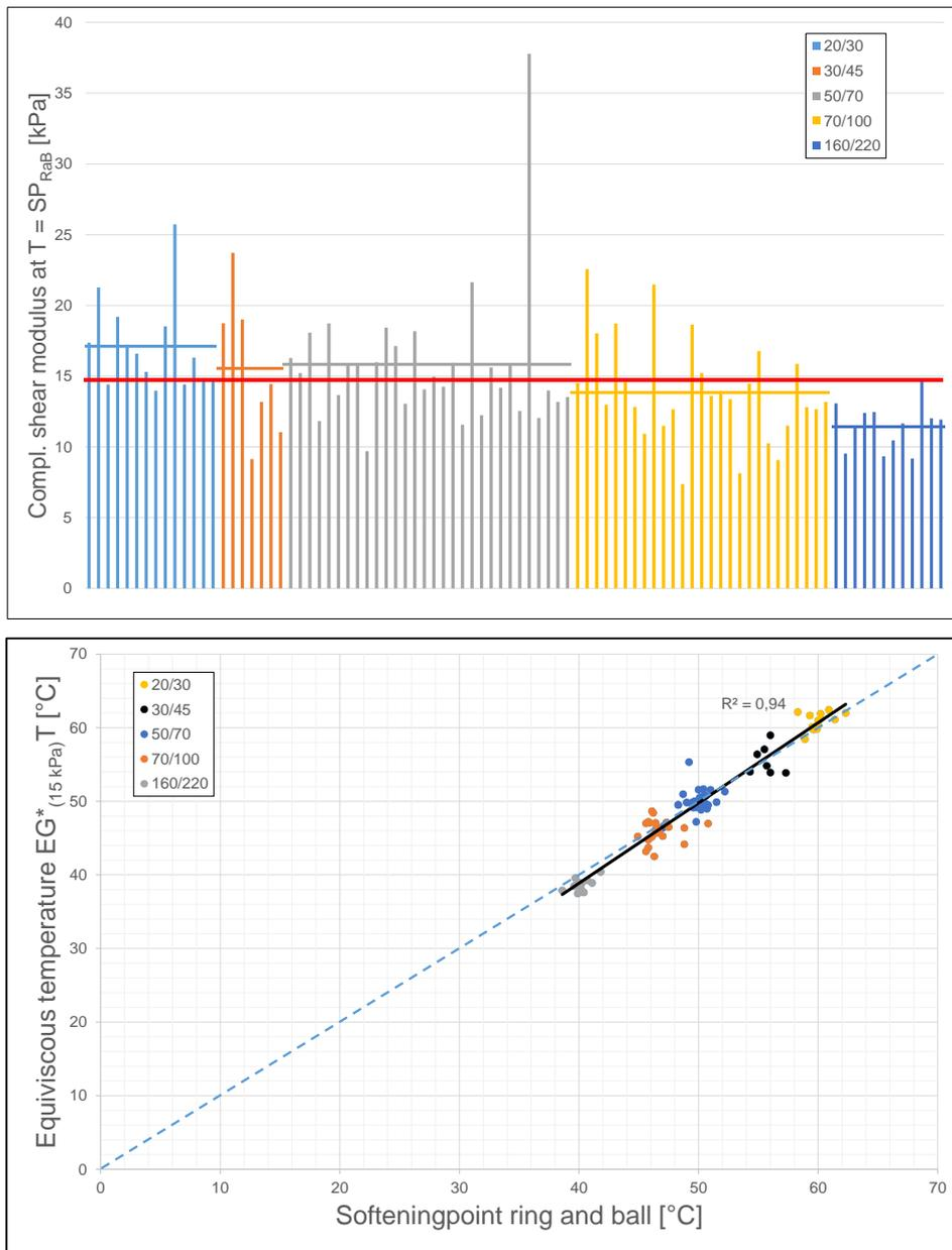
**Figure 9: Complex shear modulus at the temperature of the softening point ring and ball (top); correlation between softening point ring and ball and equiviscous temperature  $EG^*_{15kPa}T$  (down)**
