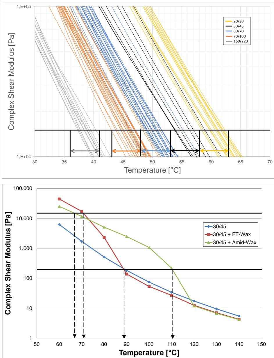
**Figure 10: Recommended limits of  $EG^*_{15kPaT}$  for each bitumen grade (top); identification of wax-modified bitumens by  $EG^*_{15kPaT}$  and  $EG^*_{0,2kPaT}$  (down)**
