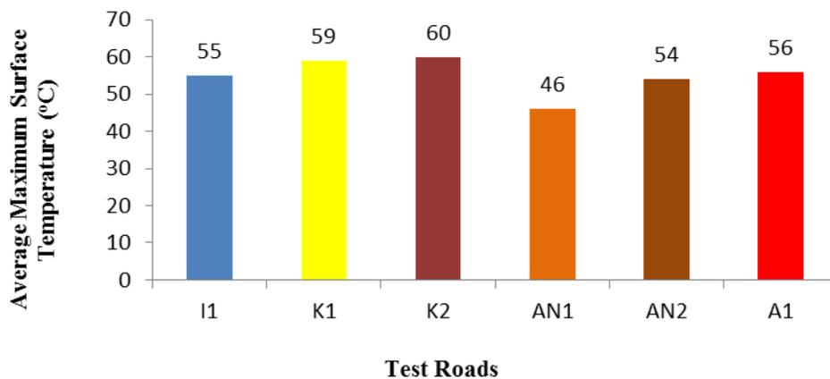
**Figure 9: Average maximum surface temperature**
