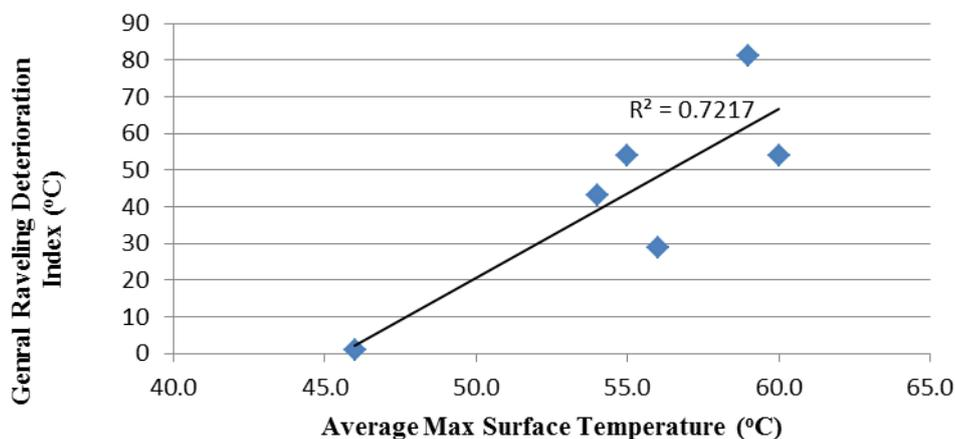
**Figure 10: Correlation between the general ravelling deterioration index and average maximum surface temperature**
