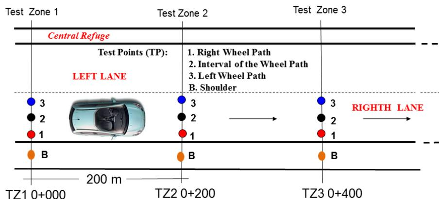
**Figure 2: Schematic plan of the non-destructive test points**
