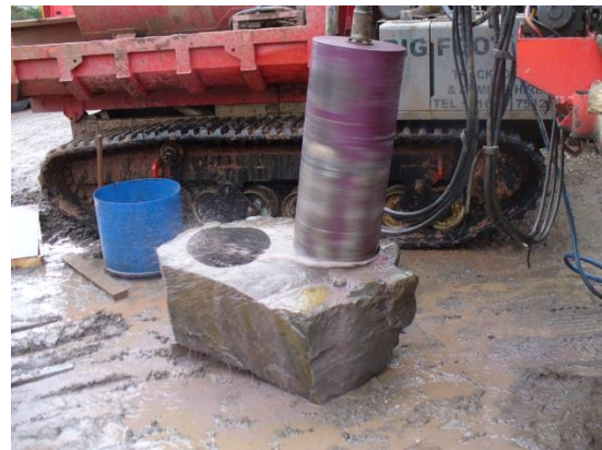
Figure 14 Coring of stone sample with a diameter of 390 mm
