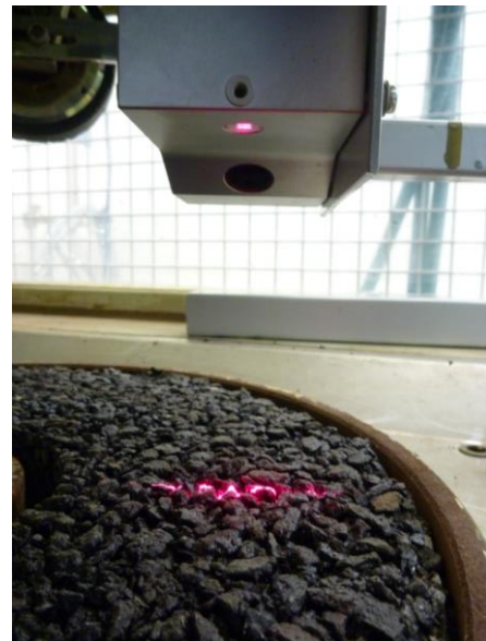
Figure 9: Scanner in SR-ITD
