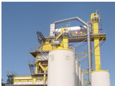
Figure 1: Batch mixing plant with parallel drum
