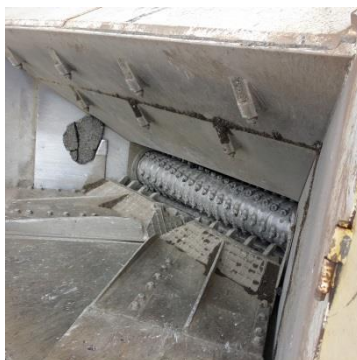
Figure 2: Special crusher for RAP
