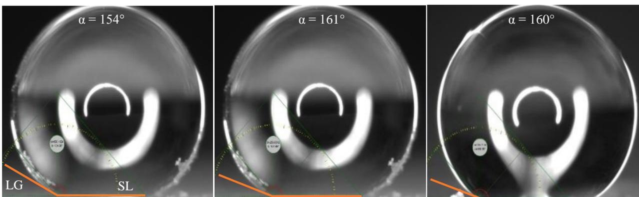
**Figure 6: An example of water contact angle measurement for three droplets deposited on one replicate**
