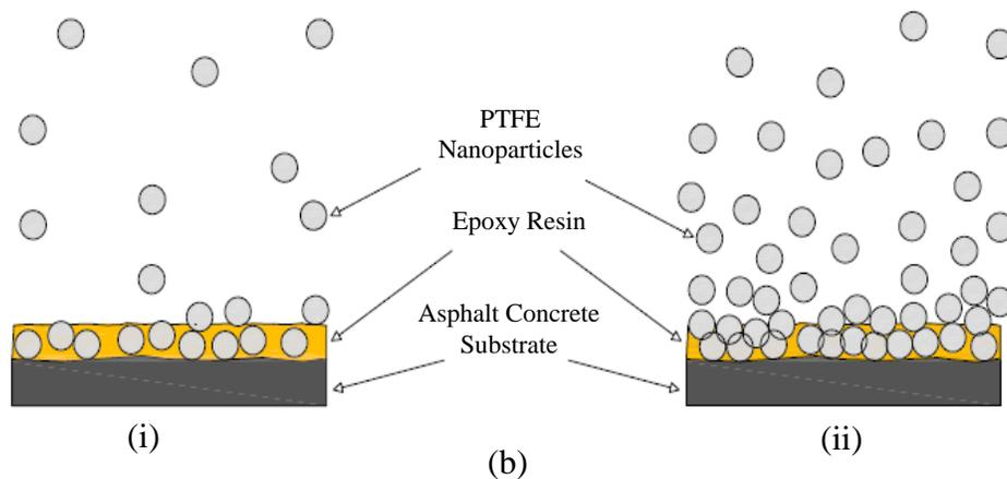
**Figure 3: Deposition of nanoparticles when the amount of PTFE is (i) low and (ii) high**
