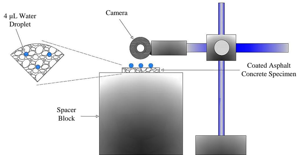
**Figure 4: Set-up used for measuring the contact angles**
