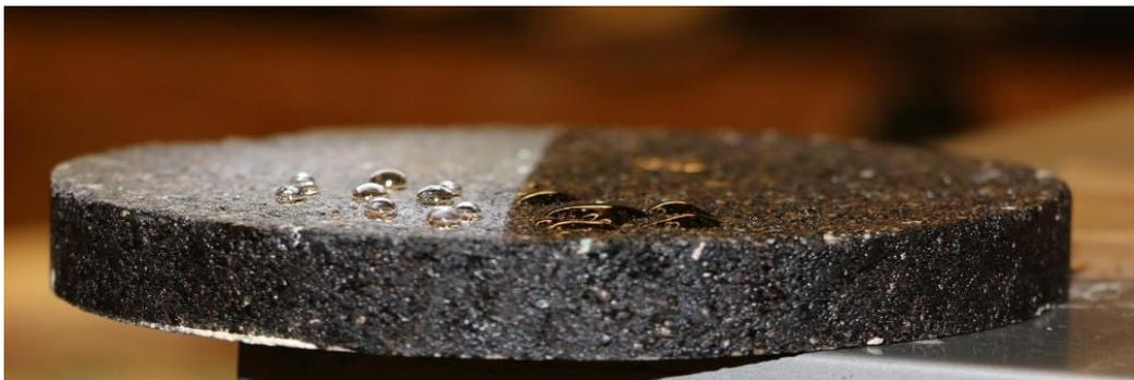
**Figure 7: The behavior of water droplet on the coated (left) and uncoated (right) cylindrical asphalt concrete specimens**
