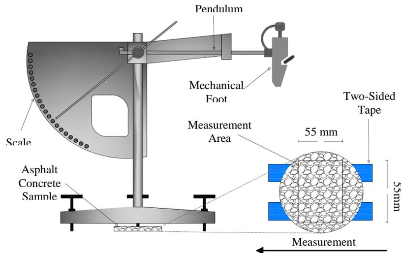
**Figure 5: Schematic of British pendulum tester**
