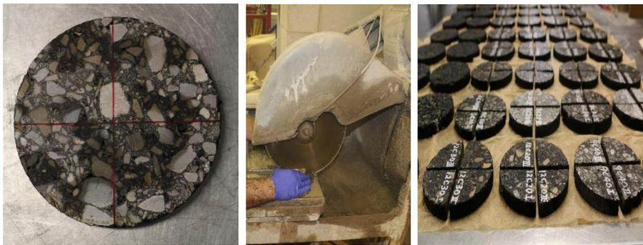
Figure 1: Preparation of asphalt concrete substrates at the laboratory
