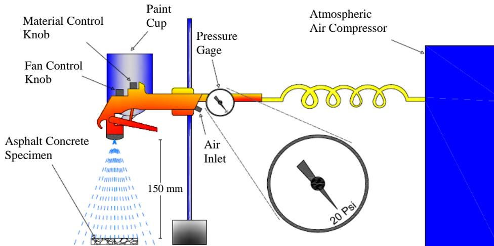
**Figure 2: Spray gun set up for spraying the epoxy and the PTFE**
