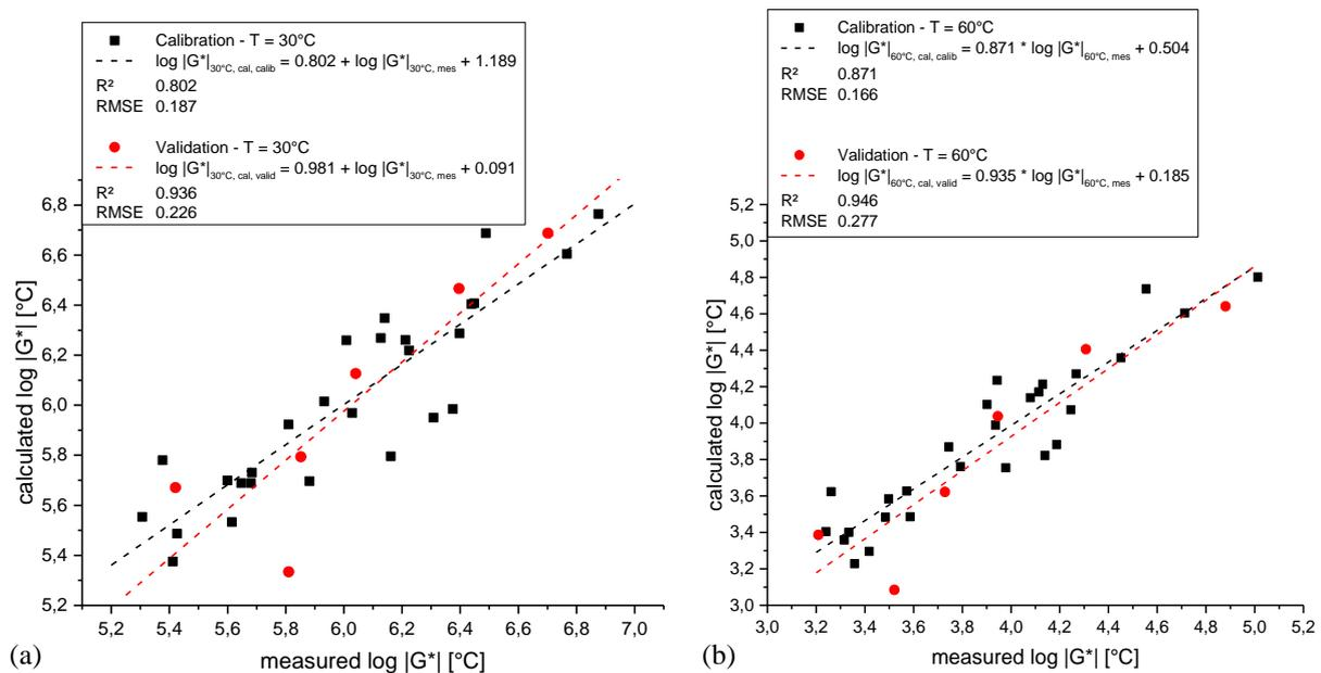
**Figure 3 Relationship between the measured and the calculated  $\log |G^*|$  at (a) 30°C and (b) 60°C as follow Table 2**
