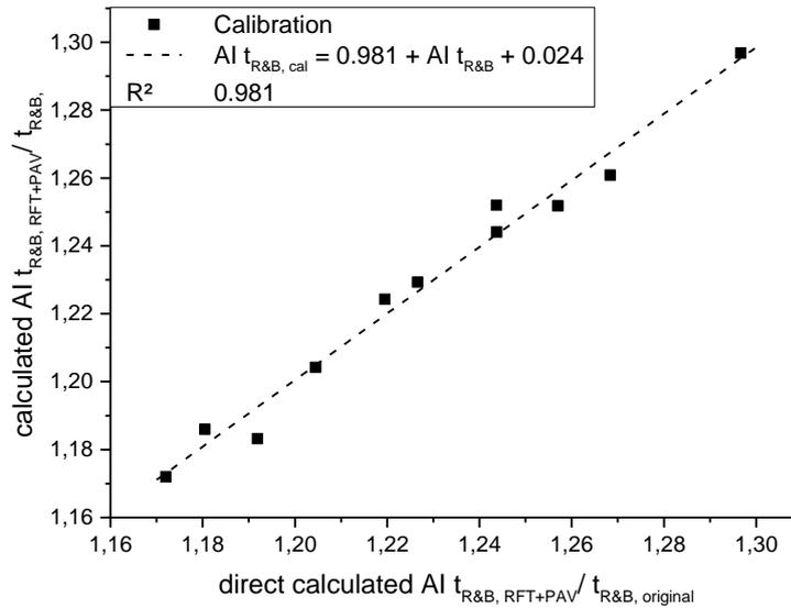
**Figure 5 Relationship between the direct from the rheological parameter calculated AI  $t_{R\&B,RFT+PAV} / t_{R\&B,original}$  and the calculated AI as follow**
