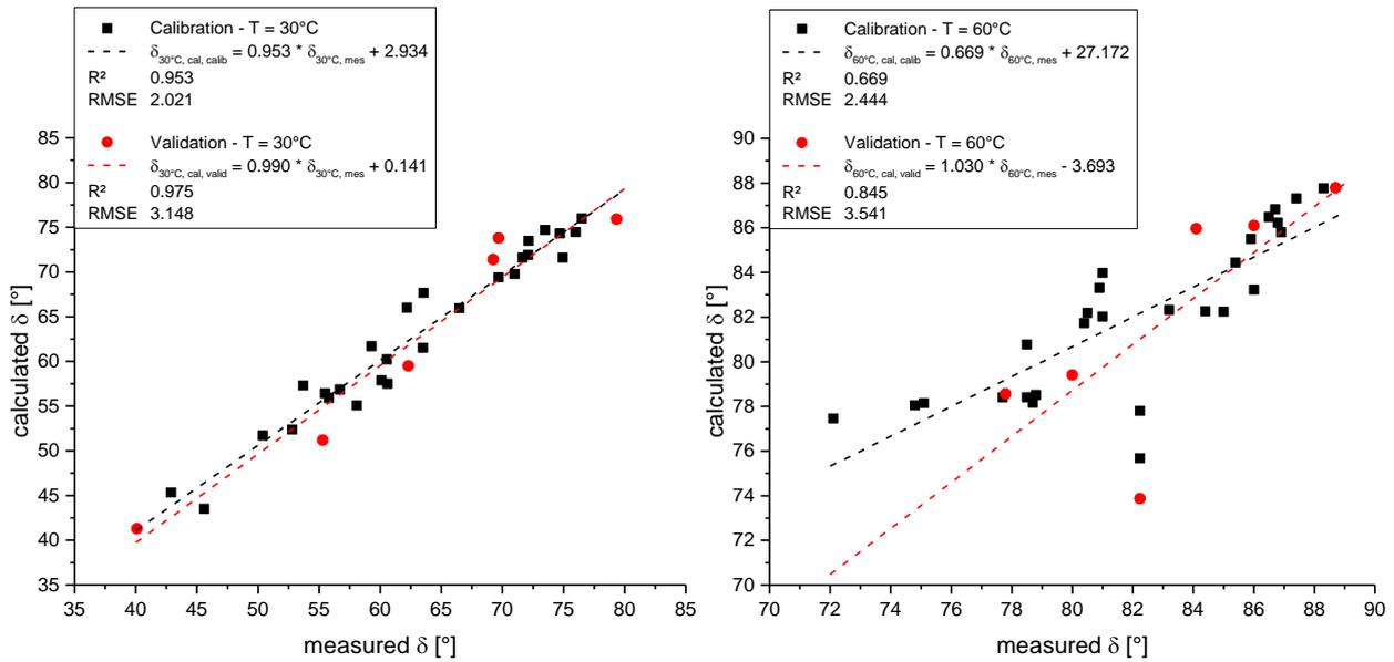
**Figure 4 Relationship between the measured and the calculated phase angle  $\delta$  at (a) 30°C and (b) 60°C as follow Table 3**
