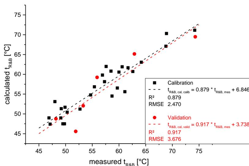
**Figure 2 Relationship between the measured and the calculated softening point  $t_{R\&B}$  as follow**
