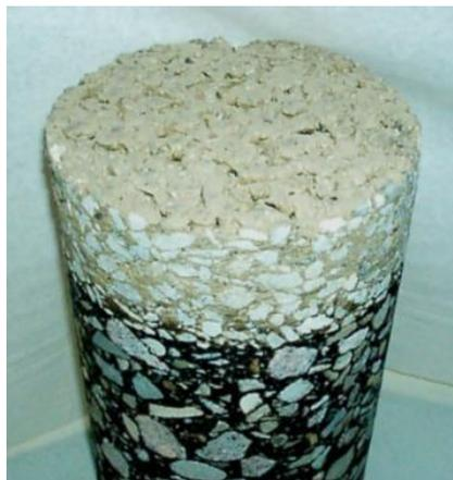
Figure 1: Light coloured asphalt
