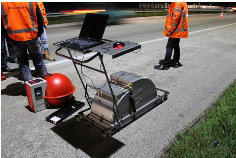
Figure 10: Night visibility at public lighting (average luminance coefficient Q0-S1-S2)
