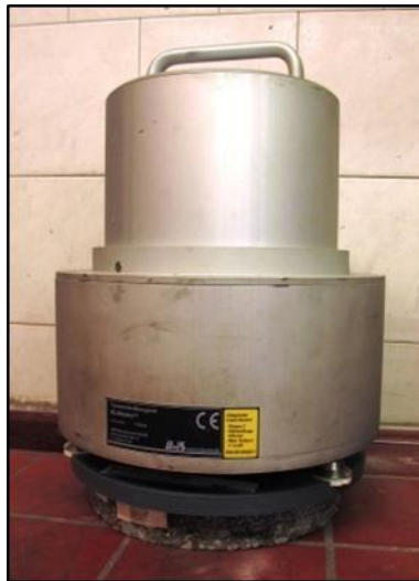
Figure 5: Modified ELAtextur ® measuring instrument
