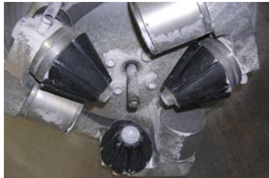
Figure 2: Testing set to EN 12697-49 polishing head
