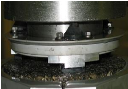
Figure 3: Testing set to EN 12697-49 measuring head
