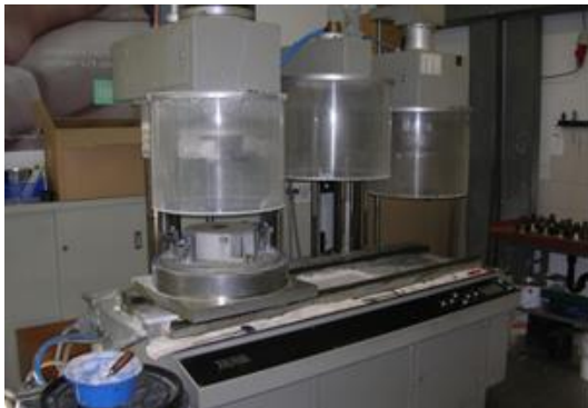
Figure 1: Testing set to EN 12697-49 for the procedure to Wehner/Schulz (polishing unit and friction measuring unit)
