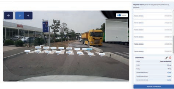
Figure 7 - Illustration of the calibration tool on a pedestrian crossing of known dimensions - a reference object commonly used by default as a checkerboard.
