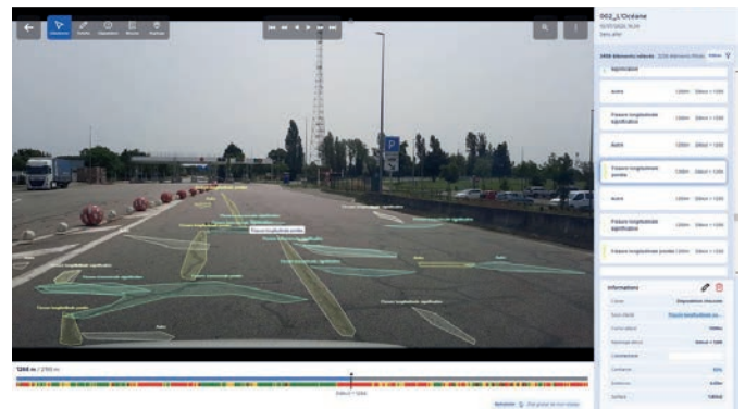
Figure 8 - Illustration of Artificial Intelligence analysis using the Roadcare Segmentation model.
