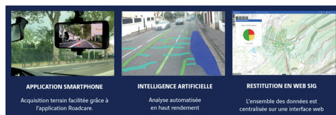
Figure 1 - How the Roadcare solution works: simplified Smartphone acquisition, automated Artificial Intelligence damage survey and GIS web platform for reporting and decision support.
