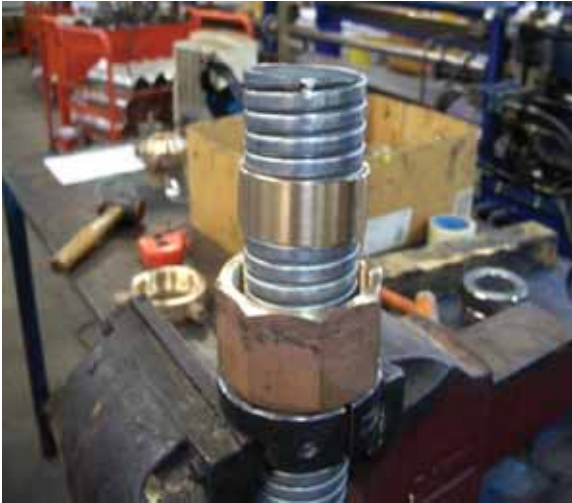
Ferrule and lock nut in place during assembly
