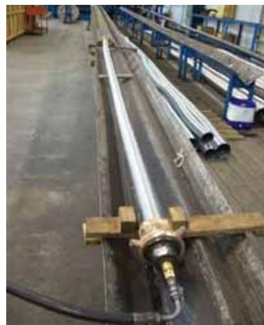
Stripwound bitumen hose being pressure tested
