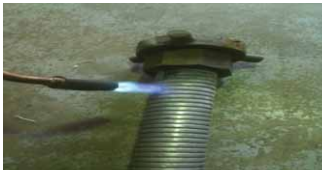
Poor practice: externally heating a hose with a gas torch
