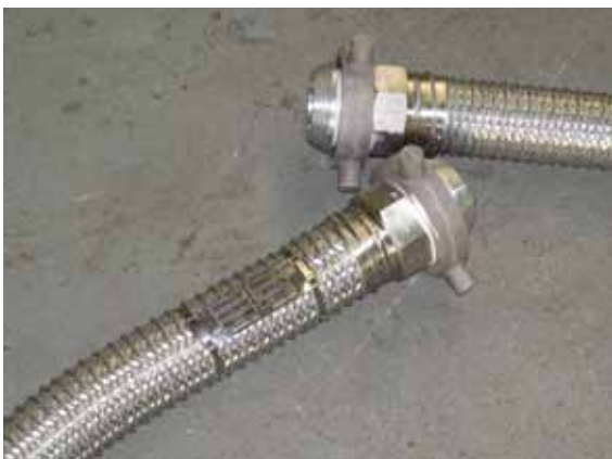
Aluminium fittings and with braid and protective armour wire applied
