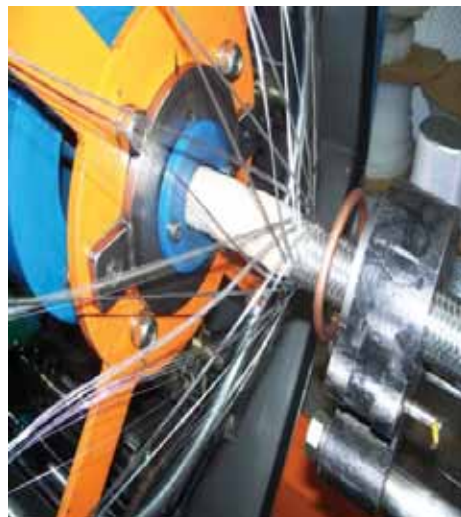
Braid being applied over top of optional insulation sleeve
