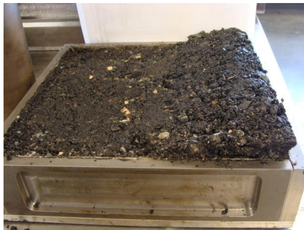
Figure 6 Mix Shoving in Mould due to RAP Agglomerates- A tender mix with agglomerated fines causes shoving in the mould
