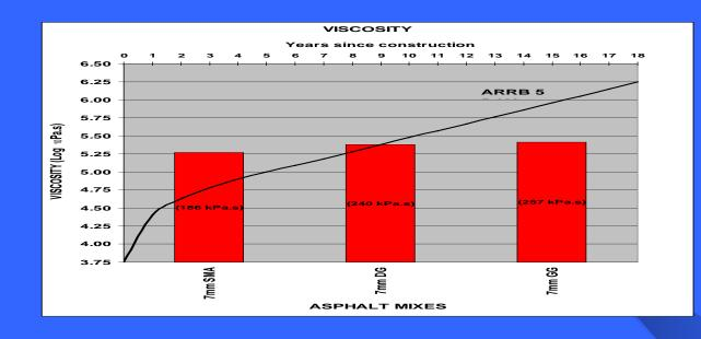
The viscosity of the SMA is lower than the dense grade and gap grade indicating that the durability of the SMA is highly likely to be better.
