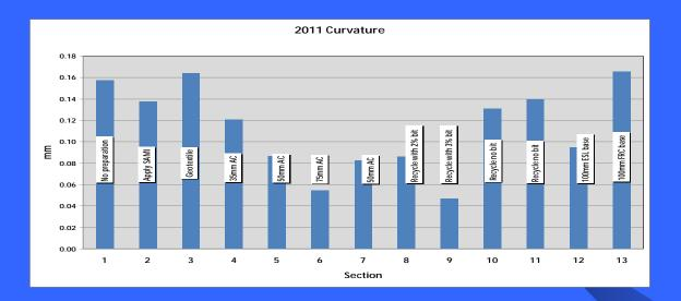
The structural capacity of the road sections that were situ recycled with the addition of 3% residual binder or constructed with 100mm of asphalt have increased such that the sections are good for classification as distributor roads with well over 1 x E6 ESA's
