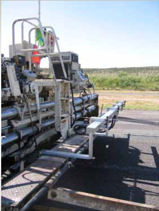
Mounts on paver – once running requires no operator
