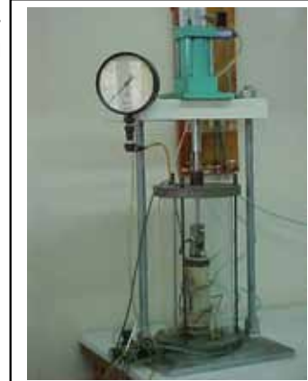
Resilient Modulus equipment for unbound materials. IMAE. University of Rosario, Argentina.
