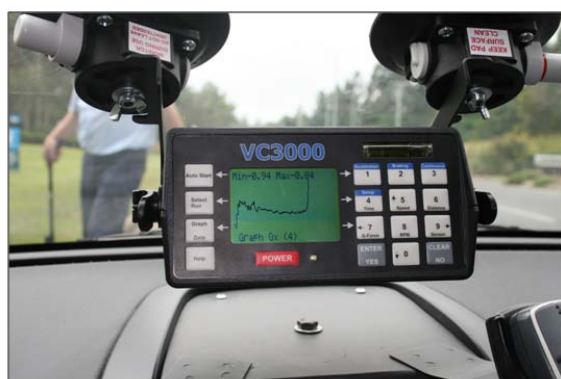
Vericom test device and output – David Tulloch, QTMR/QPS
