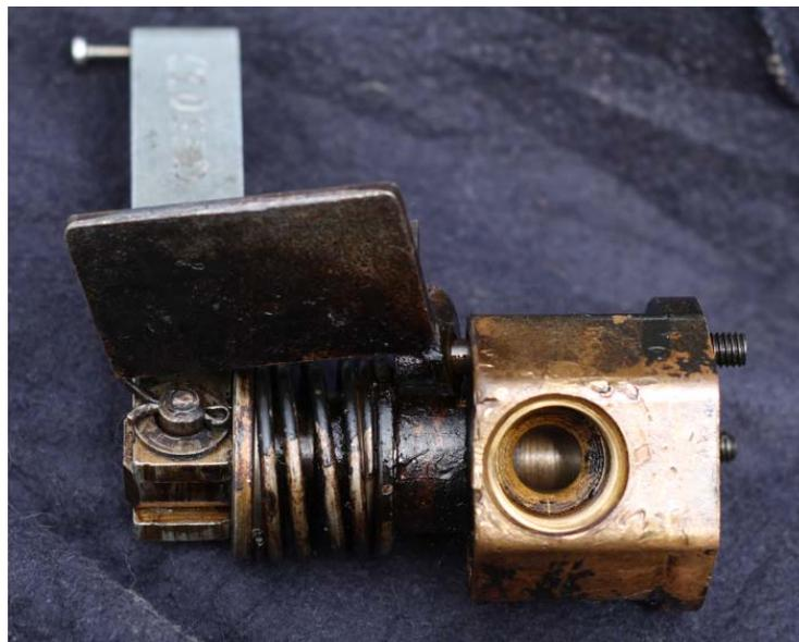
**Figure 6: Nozzle apparatus with valve open**
