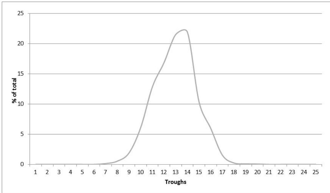
**Figure 5: Spray pattern with no nozzle**
