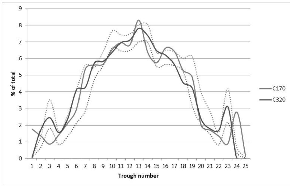
Figure 13: Spray profiles of bitumen products
