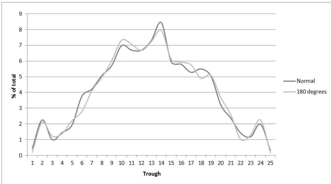
Figure 4: Nozzle J with standard and reversed orientation
