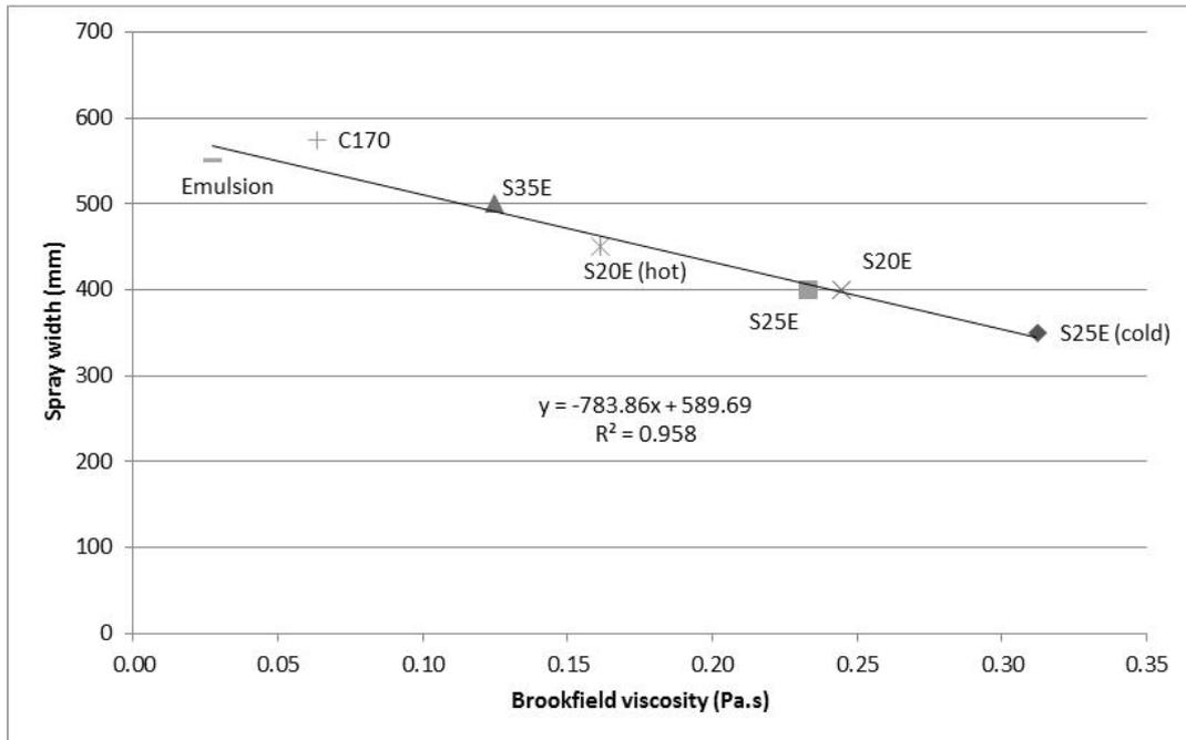
**Figure 16: Brookfield viscosity results of sprayed products**
