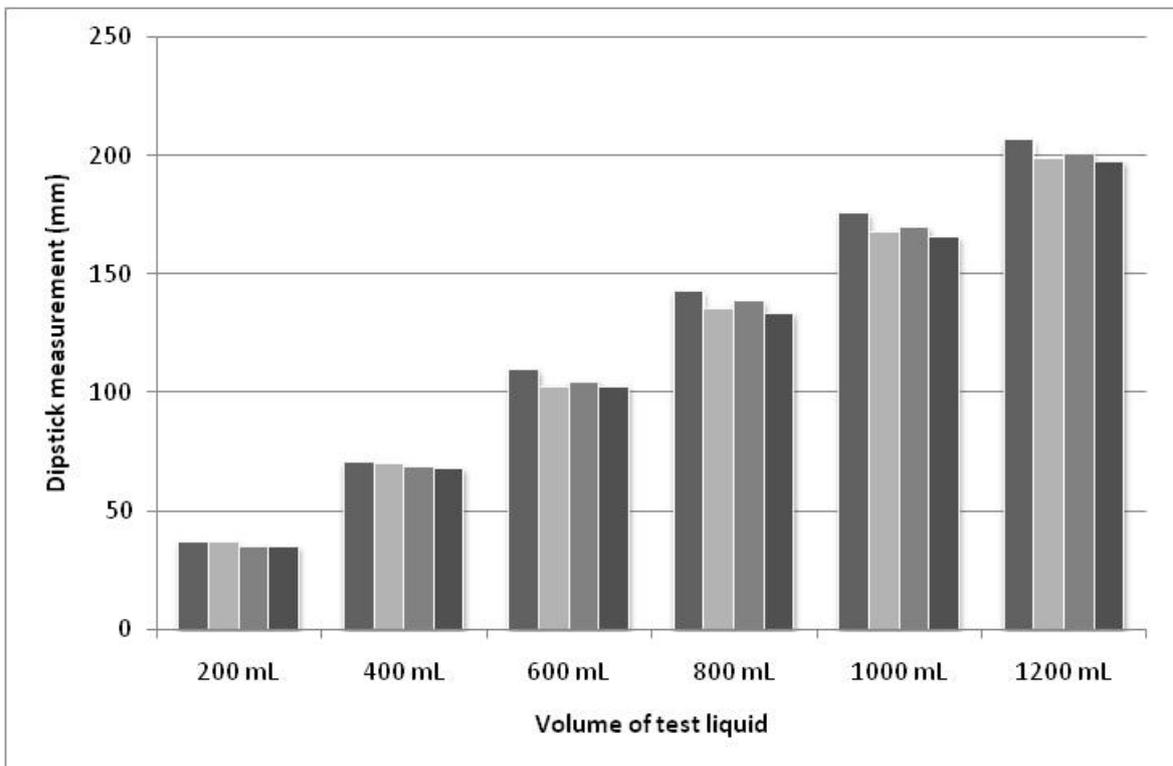
Figure 3: Dipstick measurement repeatability
