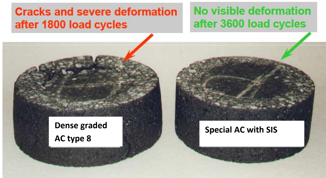
Figure 4: Comparison of asphalt concrete with and without SIS in dynamic creep test.
