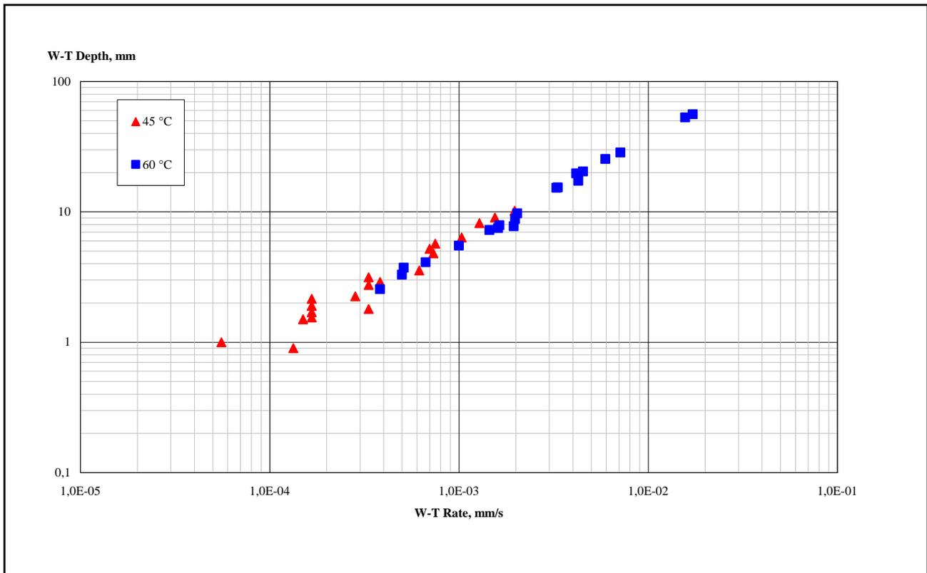
**Figure 3 : Wheel-tracking rut depth against rut rate**
