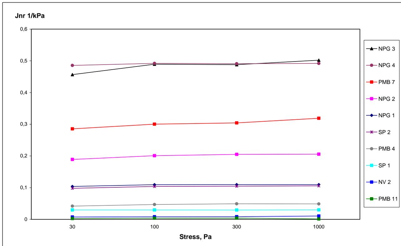
Figure 2 : Non-recoverable creep compliance  $J_{nr}$  in the range of 30 Pa to 1000 Pa (45°C)
