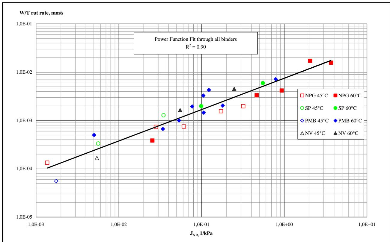
Figure 8 : Wheel tracking rut rate vs  $J_{nr}$  of RTFOT aged bitumen at 45 °C and 60 °C
