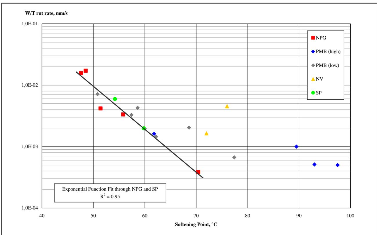
Figure 4: Wheel tracking rut rate at 60°C vs Softening Point of unaged binder
