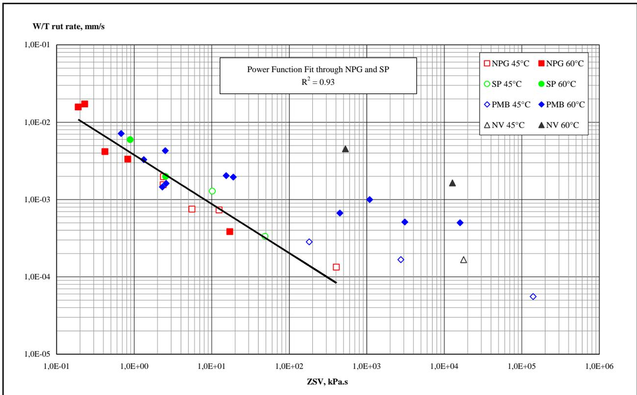
**Figure 5: Wheel tracking rut rate vs ZSV of unaged binders at 45 and 60°C**
