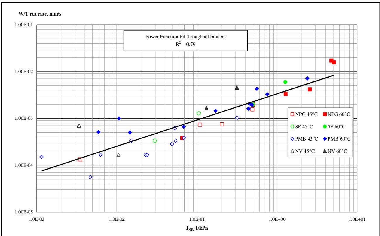
Figure 7: Wheel tracking rut rate against  $J_{nr}$  of unaged bitumen at 45 and 60 °C
