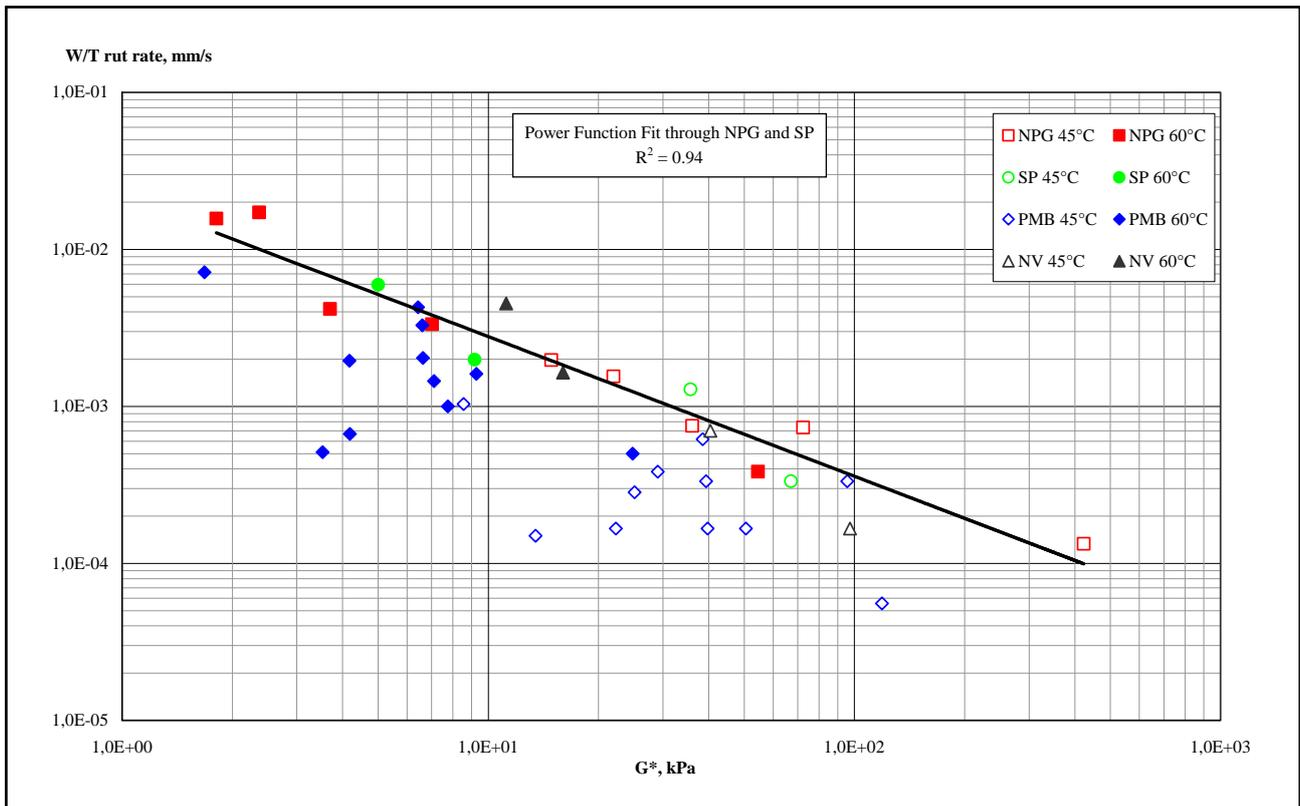
Figure 6 : Wheel tracking rut rate vs stiffness modulus  $G^*$  (1.59 Hz) of unaged binders at 45 and 60°C
