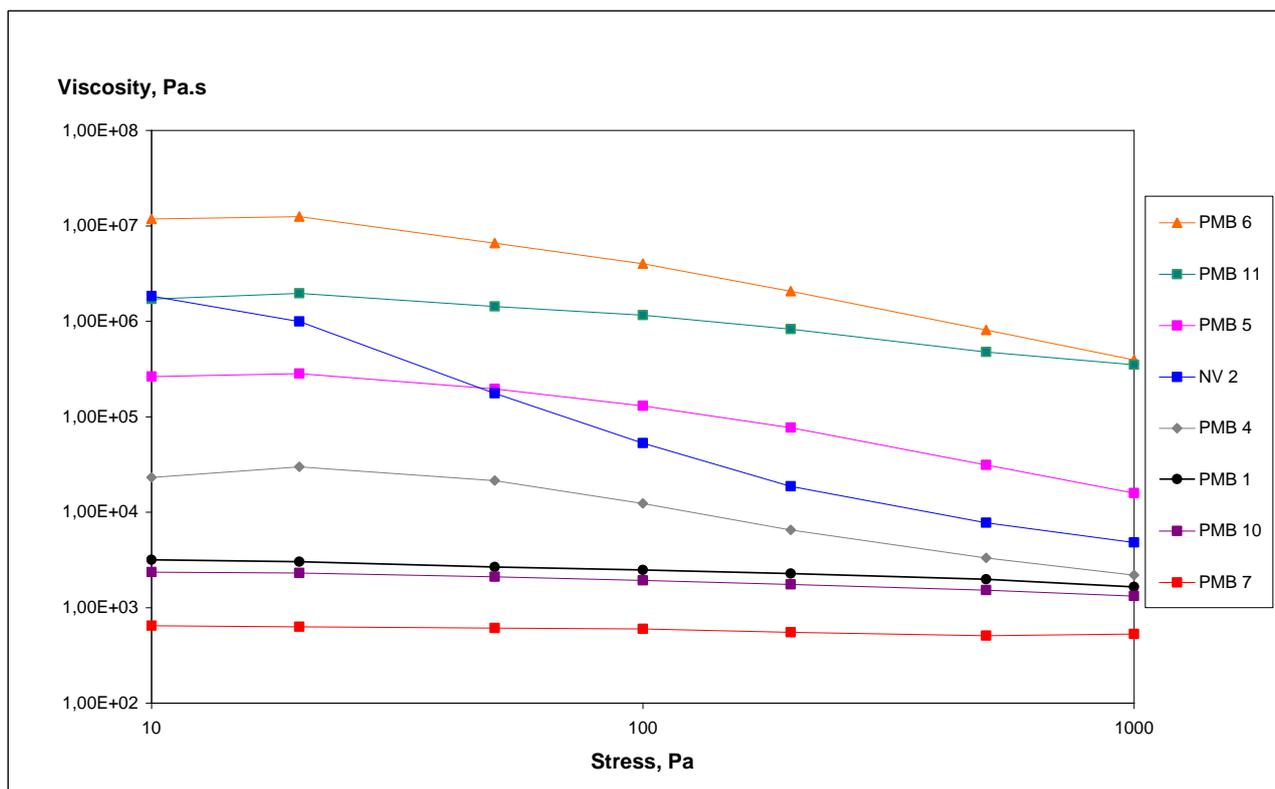
**Figure 1 : ZSV test Step 1 for polymer modified binders (60°C)**
