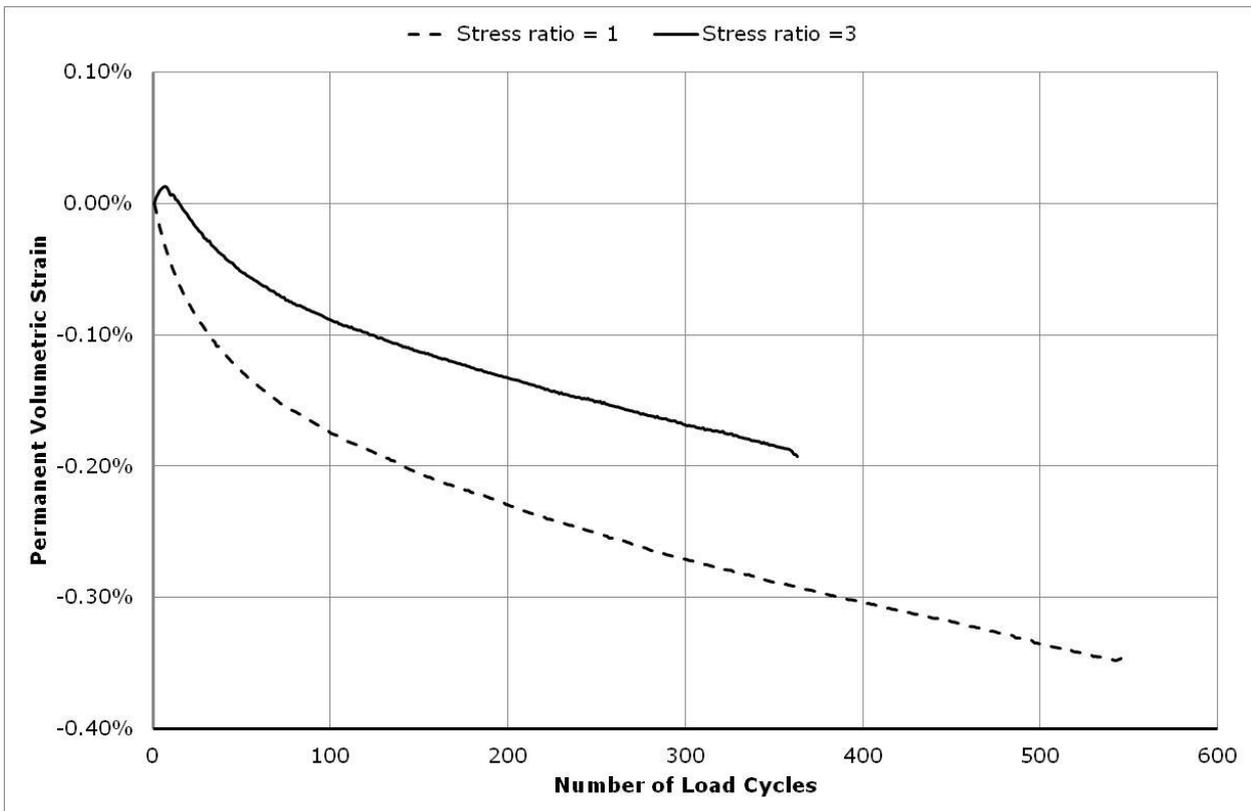
**Figure 11. Permanent shear and volumetric strain against number of load cycles at two stress ratios and a shear stress of 130kPa**
