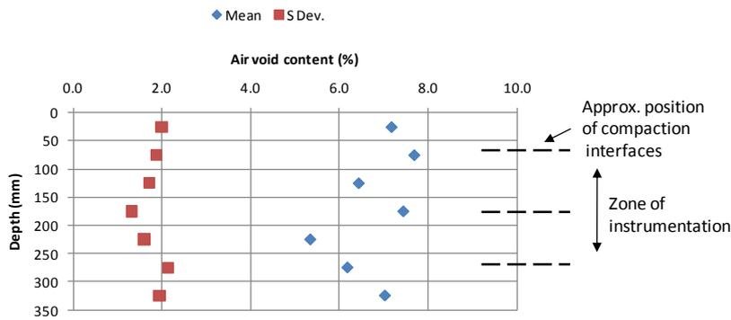
Figure 7. Mean and Standard Deviation of air void content profiles through test specimens
