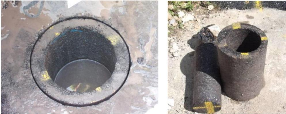
**Figure 6. Cutting of test specimens from slab**
