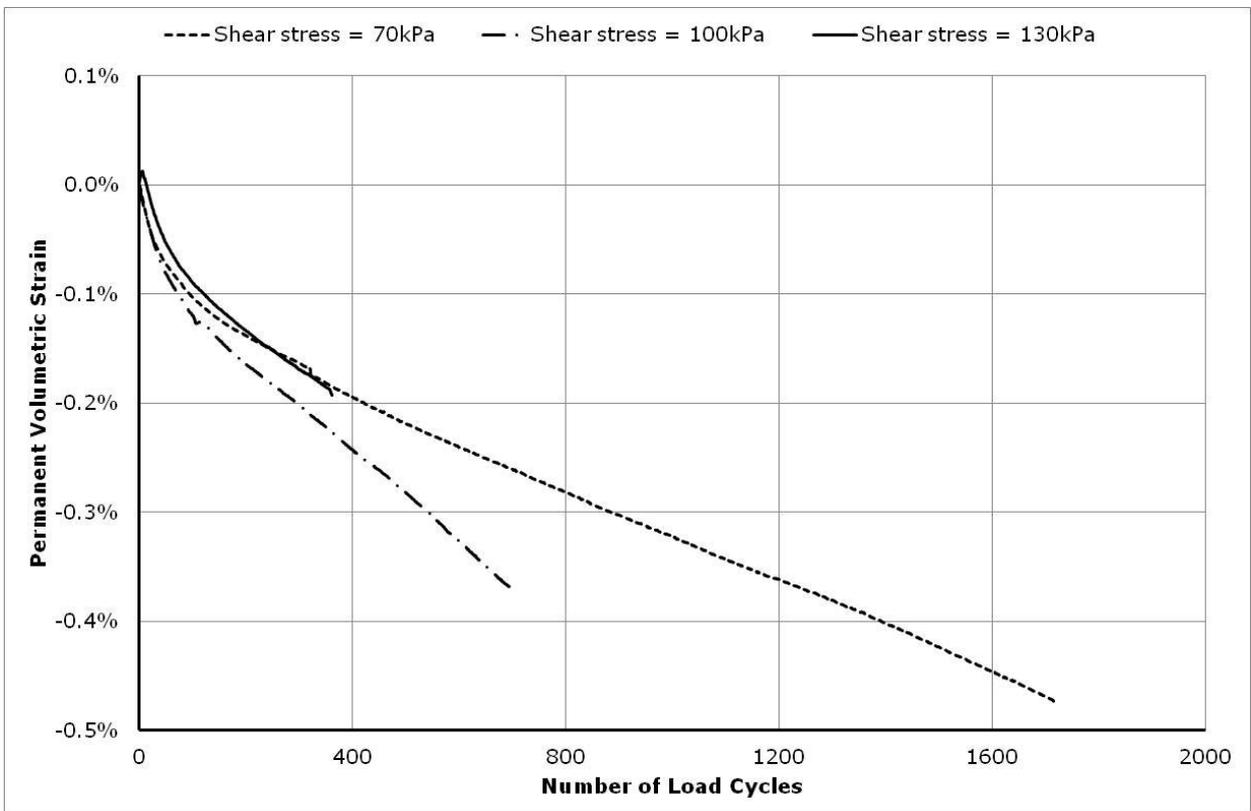
Figure 10. Permanent shear and volumetric strain against number of load cycles at three shear stress levels and a stress ratio of 3
