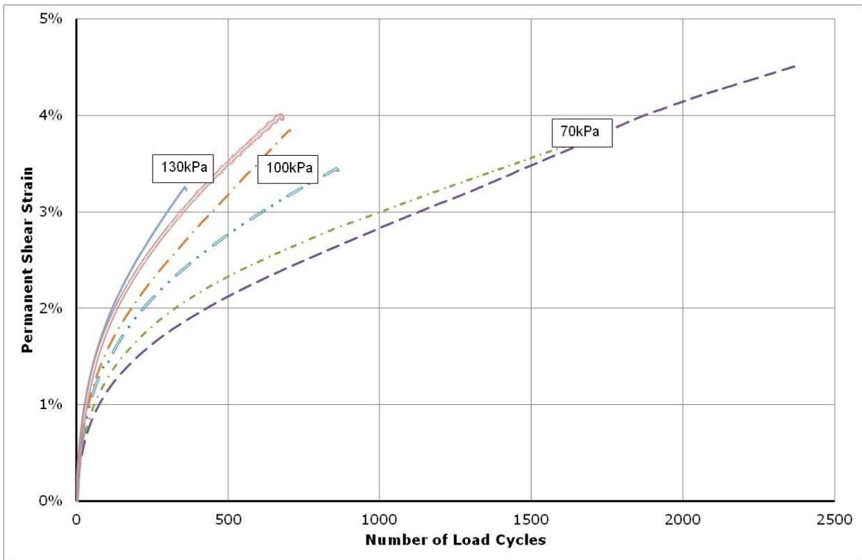
**Figure 12. Data for the individual tests illustrated in Figure 11 for shear strain**
