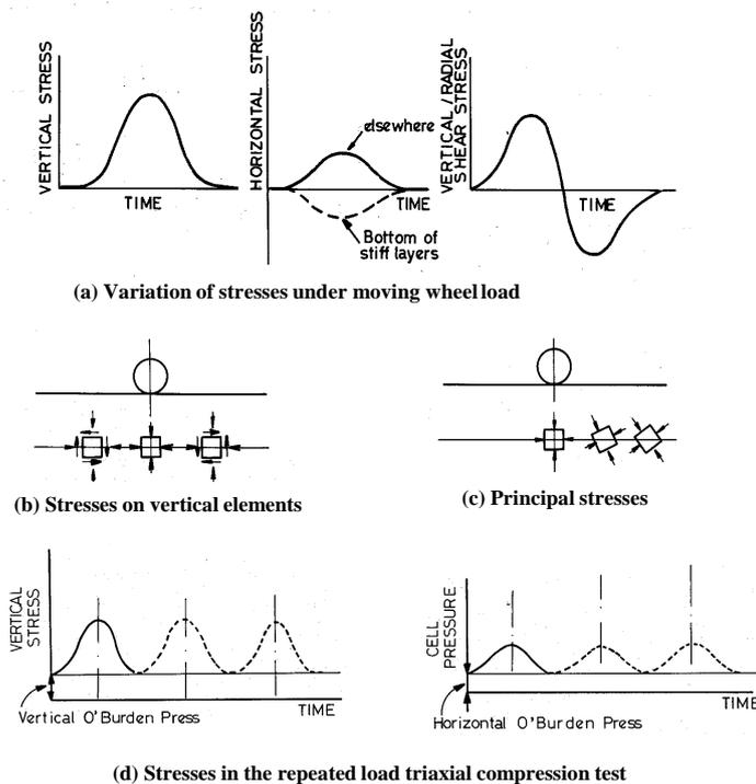
**Figure 1. Stress regimes under a moving wheel and in a triaxial test (after Pell and Brown, 1)**
