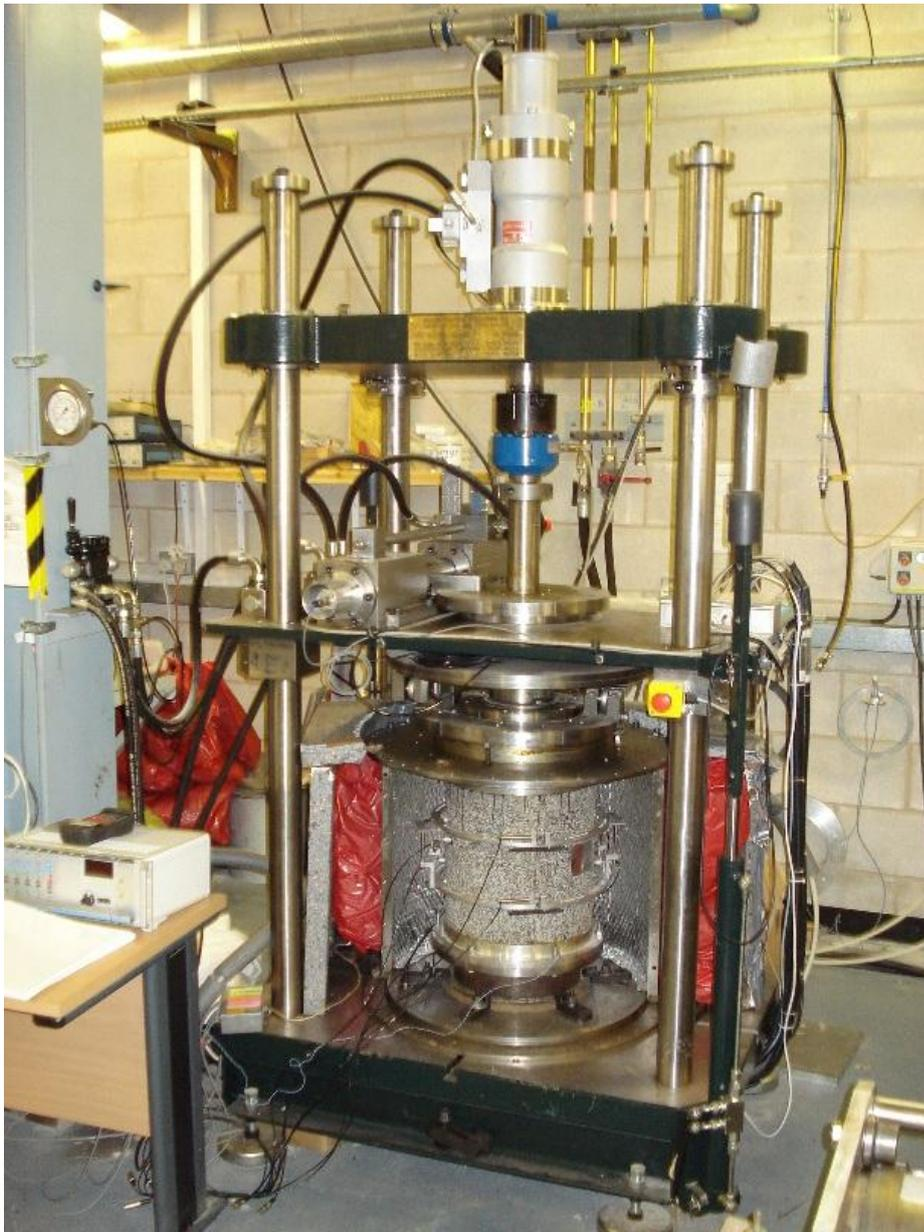
**Figure 4. HCA with test specimen in position and pressure chamber open**
