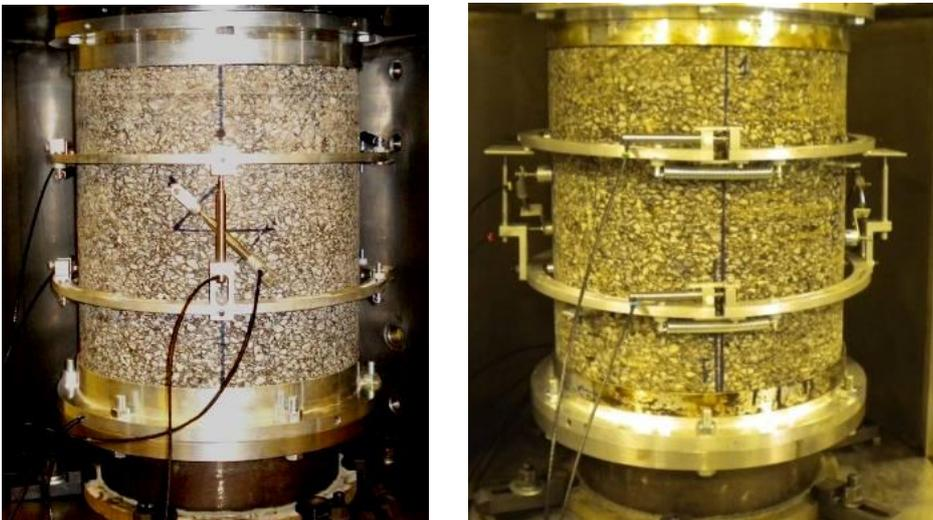
**Figure 5. LVDT displacement transducers**
