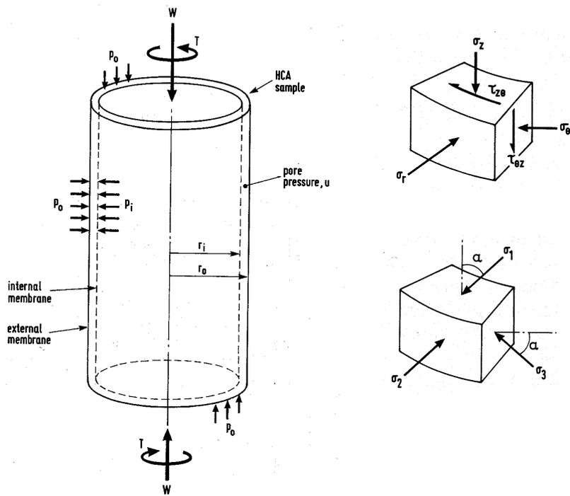
Figure 2. Schematic of a torsional hollow cylinder specimen
