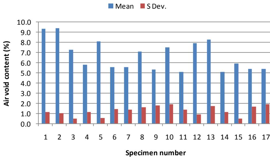
Figure 8. Mean and Standard Deviation of air void content over the instrumented sections of 17 test specimens
