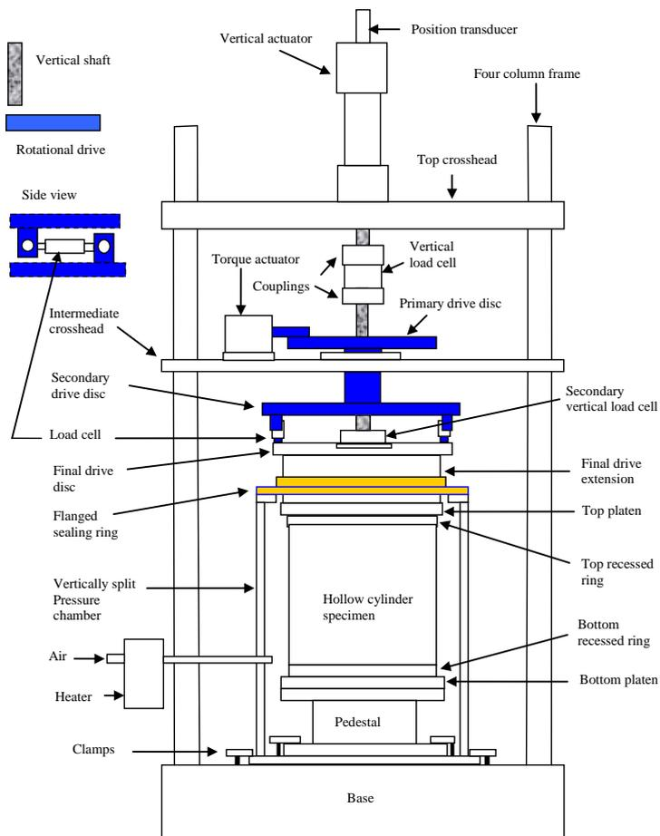
Figure 3. Cross section of Hollow Cylinder Apparatus showing principal component
