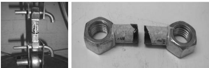
**Figure 5:** Aggregate pin drilled out from aggregate rock and stuck together with bitumen film: direct tensile test (left), and fractured pin after testing (right).
