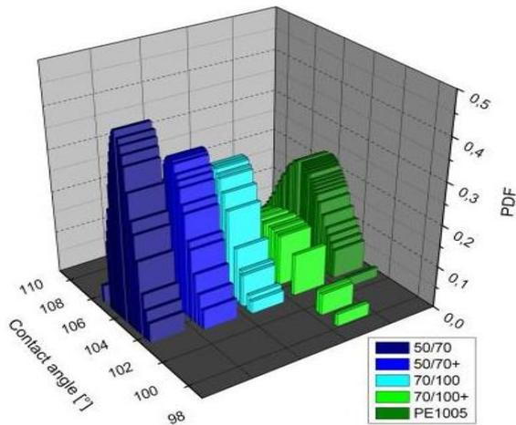
**Figure 7:** Contact angle of a water drop on bituminous surface - probability density function (PDF) plot of non-distinguishable samples
