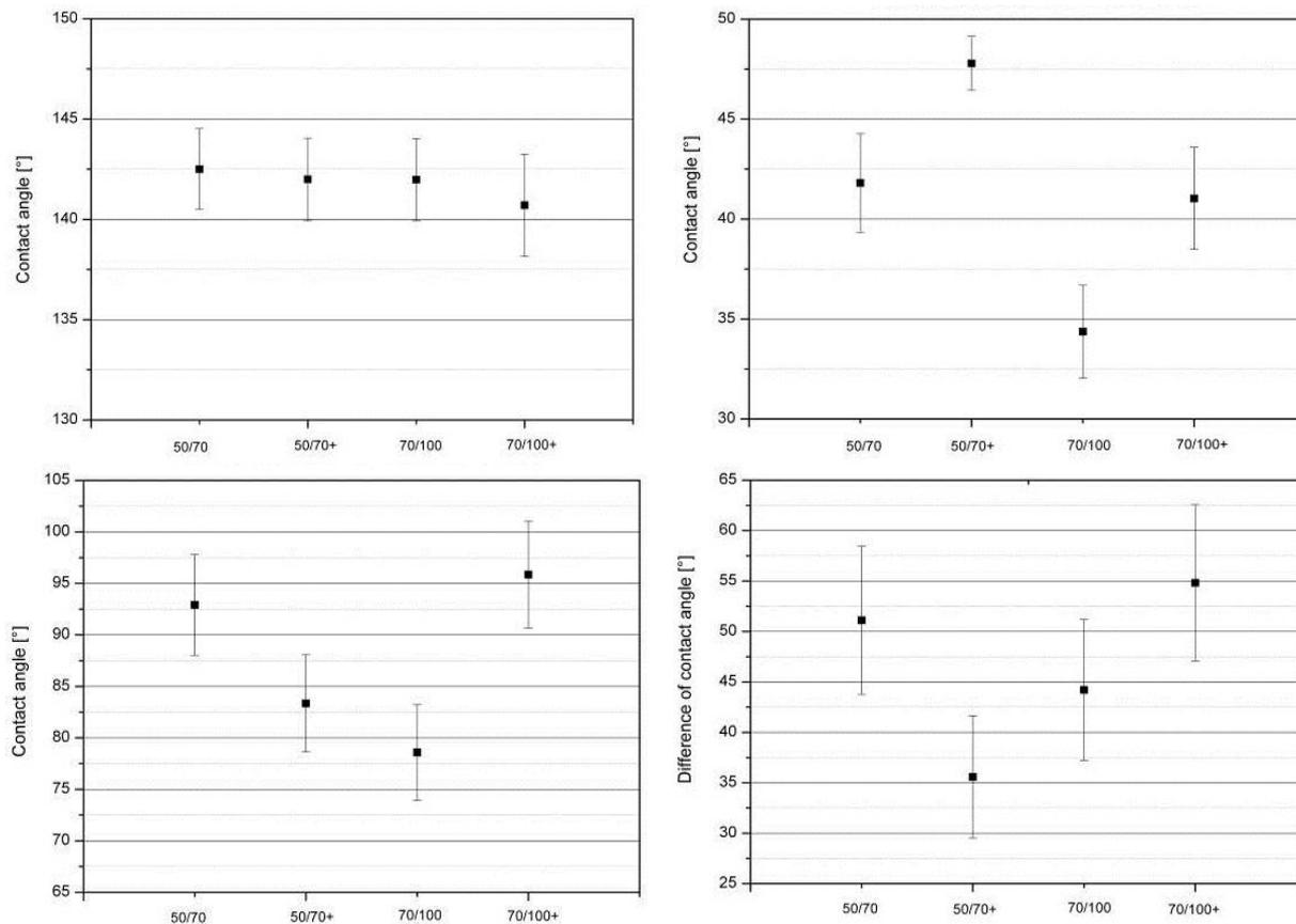
**Figure 10:** Contact angle of a bitumen drop on glass before (top left), after 30 minutes of dry storage at 70°C (top right), after water storage for 30 minutes at 70°C (bottom left), and the difference of contact angle (bottom right) for 20 samples each
