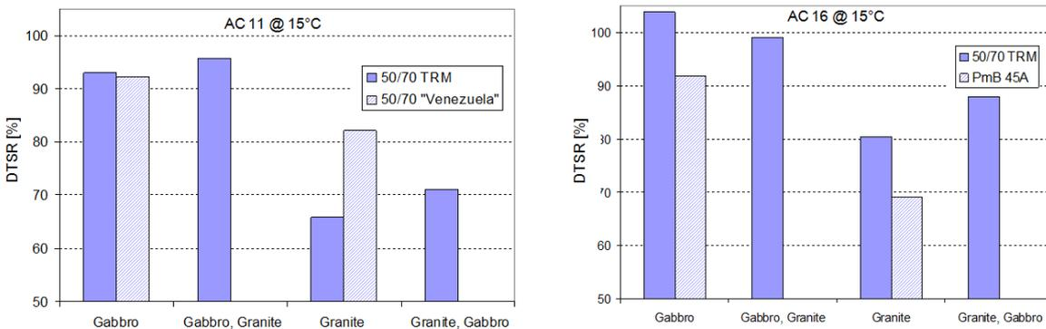
Figure 15: Influence of aggregate and bitumen type on remaining tensile strength after water storage.
