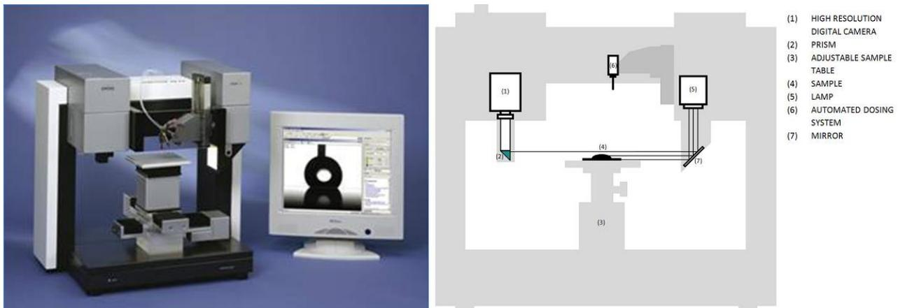
**Figure 1:** Photograph of DSA100 (KRÜSS Ltd., Hamburg, Germany) (left) and schematics of the experimental setup (right)
