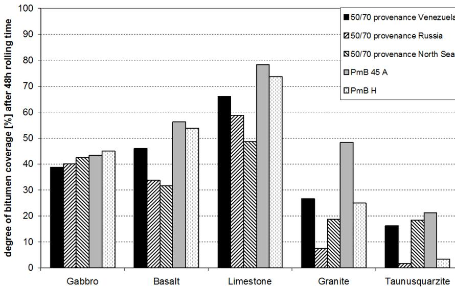
**Figure 11:** Rolling Bottle Test: degree of bitumen coverage [%] after 48 hours of rolling time
