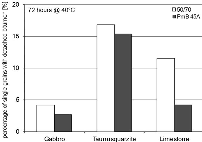
**Figure 12:** Static water storage: percentage of single grains showing detachment of bitumen
