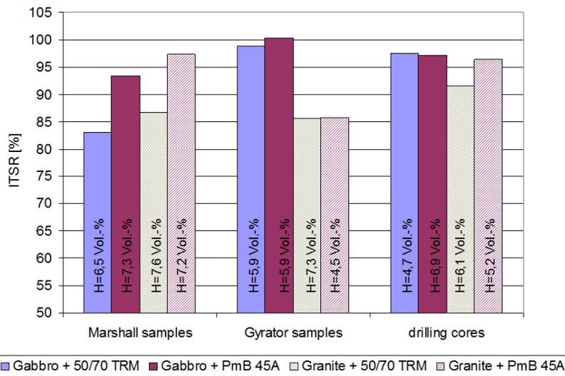
Figure 13: Indirect tensile strength test results for AC 16 at 15°C temperature: influence of bitumen type
