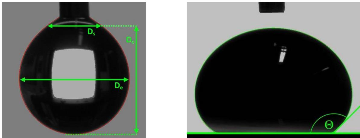
**Figure 2:** Image analysis of a hanging drop (left), and image analysis of a sessile drop (right):  $D_e$  maximum drop width,  $D_s$  parameter for drop shape ( $D_s = 0$  for exactly spherical drops),  $\Theta$  contact angle
