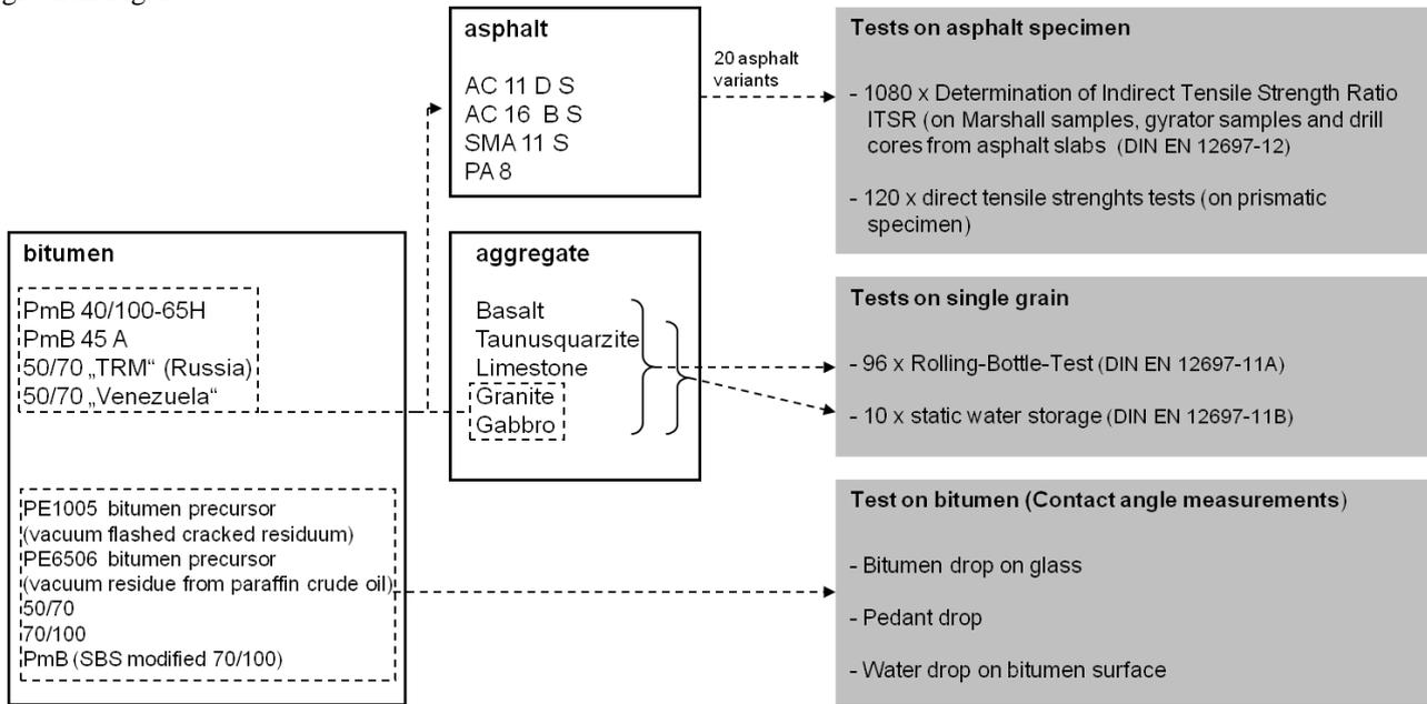
**Figure 6:** Bitumen, bitumen-aggregate combinations and asphalt mixture types assessed by the related test methods.
