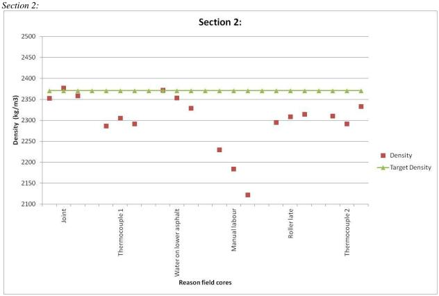
Figure 6: Density of different cores in different situation (section 2).
