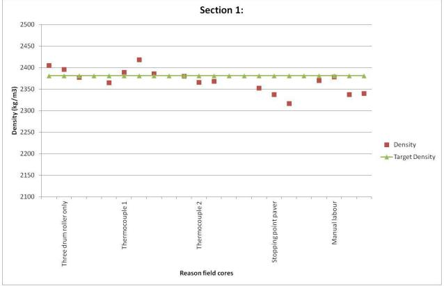
Figure 5: Density of different cores in different situation (section 1).
