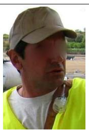
Fig. 3: the recommended position of the sampler and the adsorbent tube.
