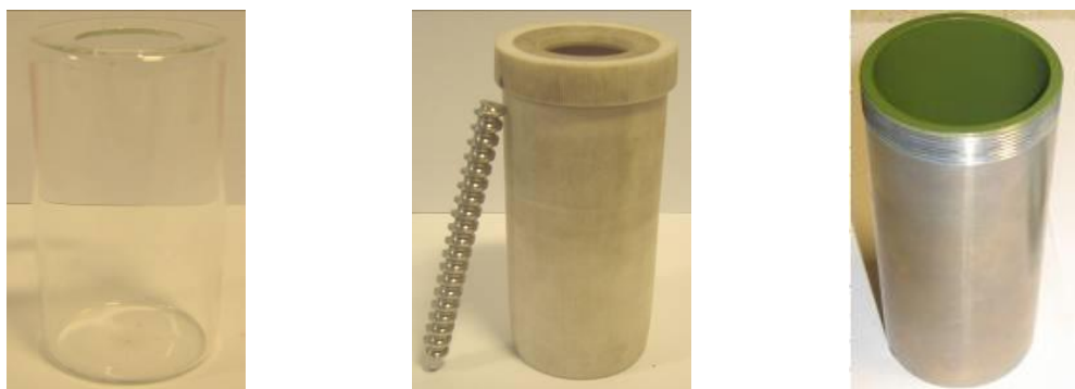
Plate 1: Glass bottle, PTFE bottle and mixing screw and “new” PTFE coated aluminium bottle (left to right)
