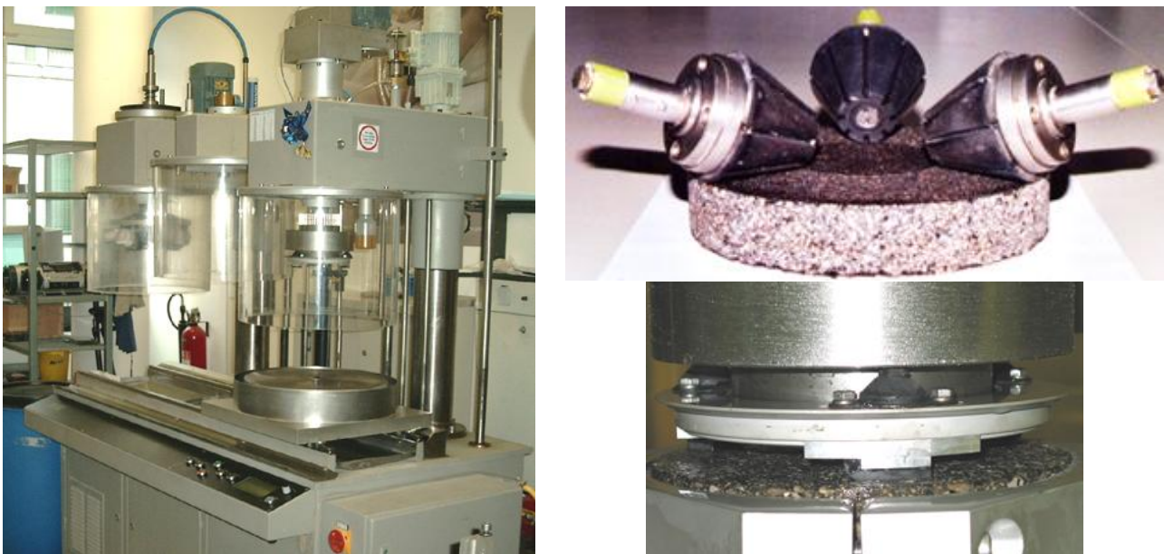
Figure 1: Test device for Wehner/Schulze (left: apparatus; right: upper picture: polishing rollers; lower picture: skid resistance measuring device)
