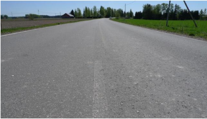
Figure 6: Iitti test road: Biofluxed binder on the left and V1500 on the right.
