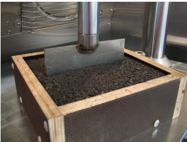
Figure 4: Blade resistance test
