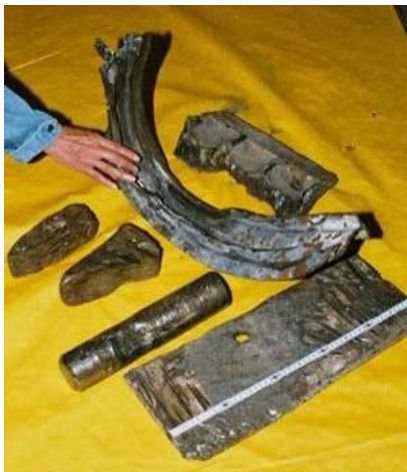
Figure 4: Steel parts, passed the primary Granulator without any damage to the machine
