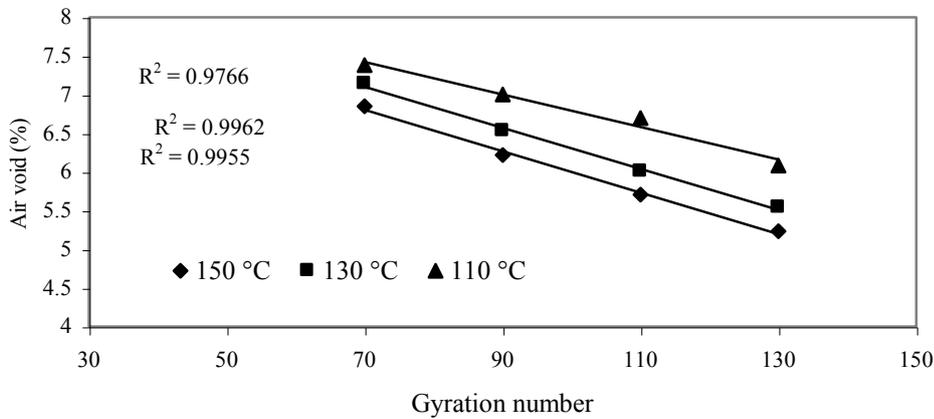
**Figure 7: The variation on air voids of gyratory compacted samples**
