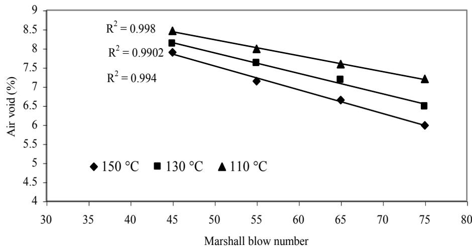
**Figure 5: The variation on air voids of Marshall hammer compacted samples**
