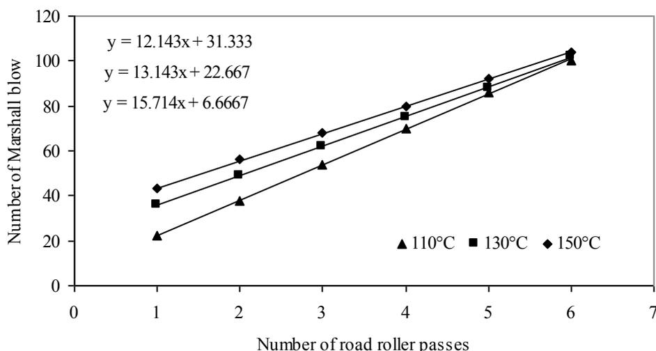
**Figure 9: The relation between Marshall blows and roller passes**
