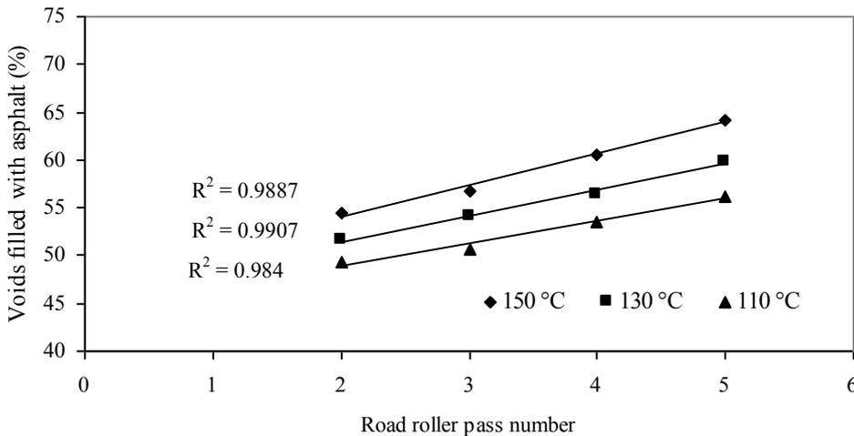
**Figure 4: The variation on VFA of core specimens**
