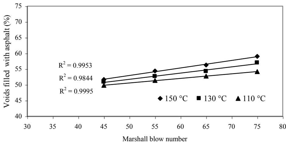
**Figure 6: The variation on VFA of Marshall hammer compacted samples**
