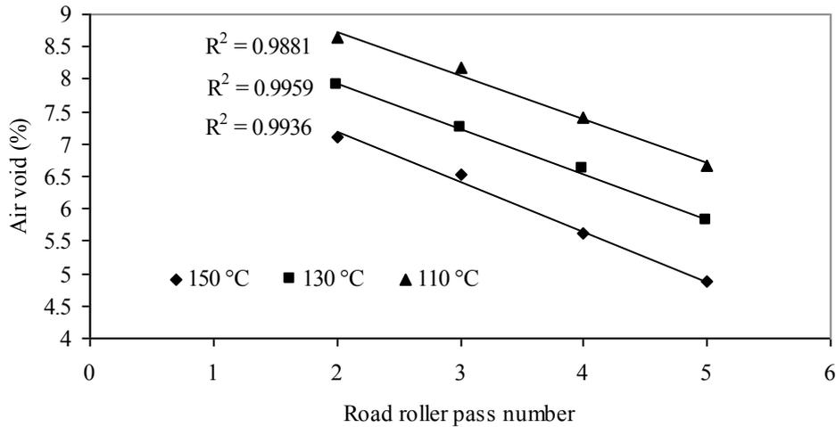
**Figure 3: Variation on air voids of core specimens.**
