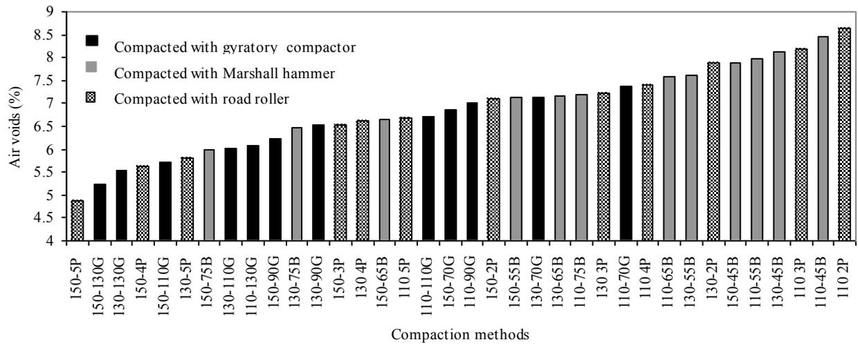
**Figure 11: The relation between the air voids and compaction methods**
