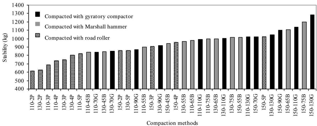
**Figure 12: The relation between the stability and compaction methods**
