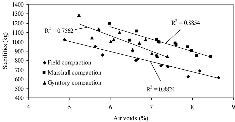
**Figure 13: The relationship between the air voids and stability**
