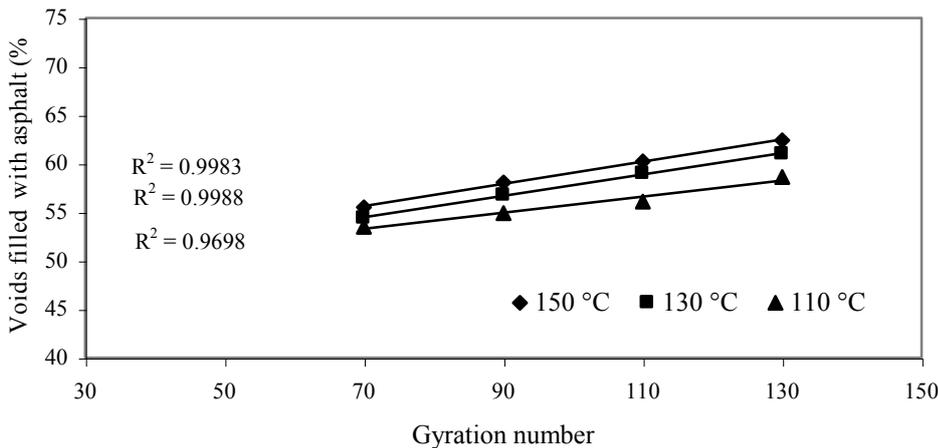
**Figure 8: The variation on VFA of gyratory compacted samples**
