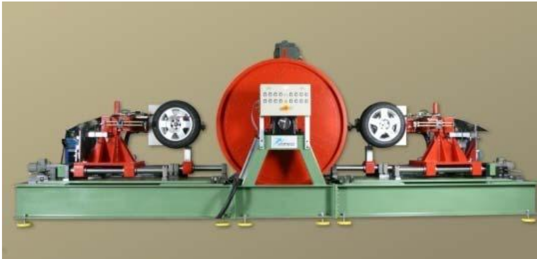
Fig.7: Steel drum test machine for tyre testing (ref. 6)
