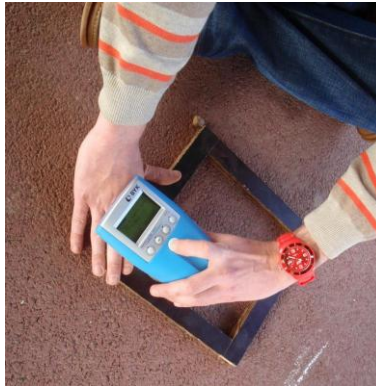
Figure 9: Per area of 20 cm by 20 cm, 4 measurements are made: one in each corner of a wooden frame.
