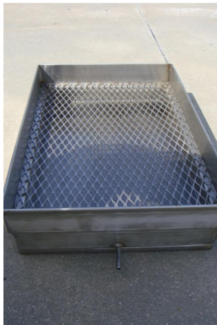
Figure 5: Collection Trays used for each slab in the APWS
