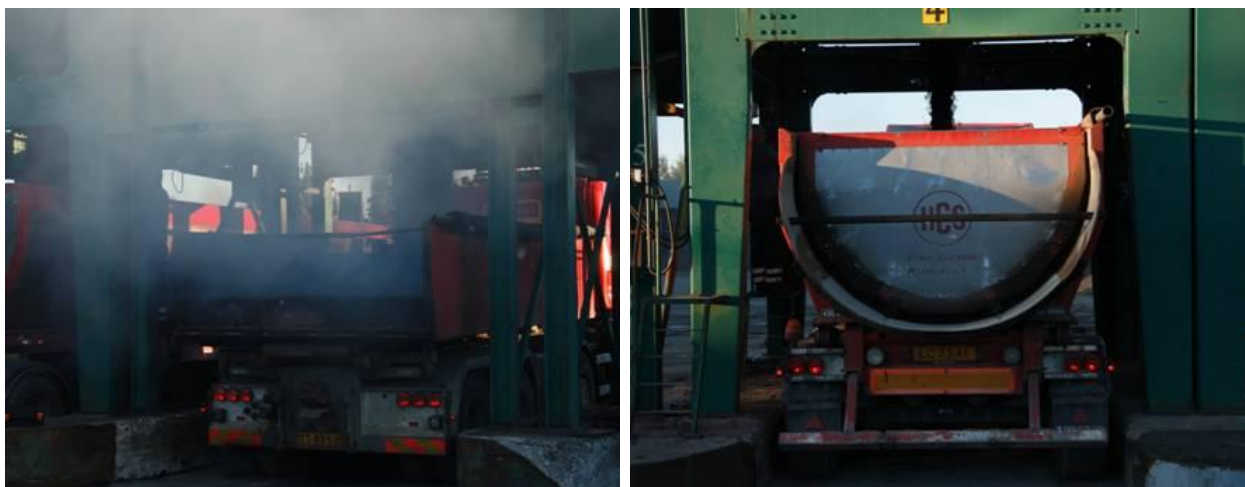
Figure 2 Fumes generates during truck loading. Left HMA, Right WMA
