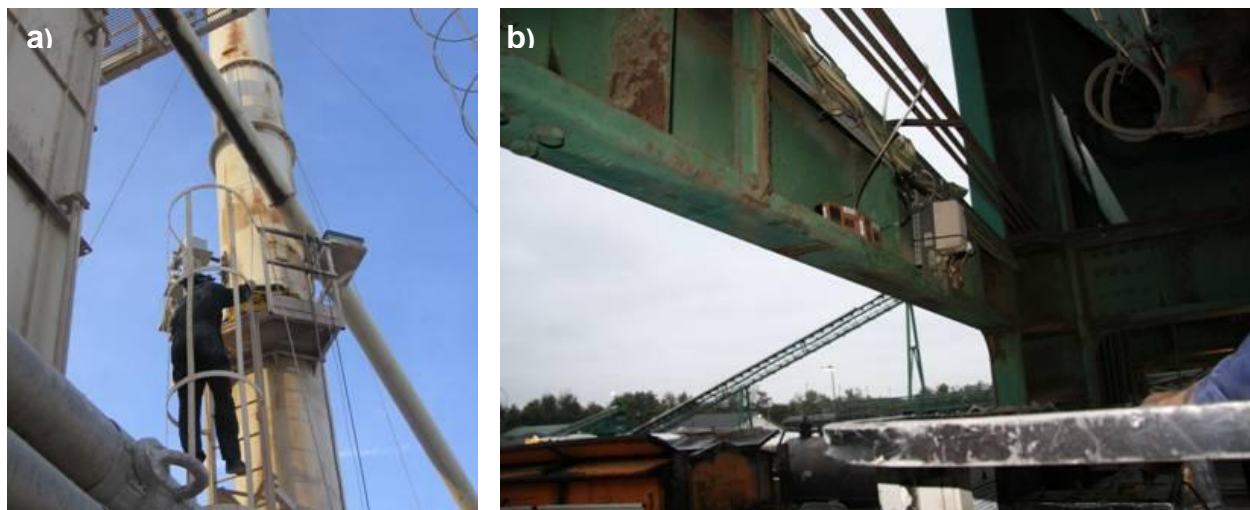
Figure 1 Placement of air emissions detectors on the chimney for the BBTM (a) and on top of the truck loading station for the SMA (b)
