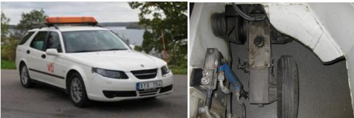
Figure 6: VTI's friction measurement car with the braked measuring wheel located under the car.
