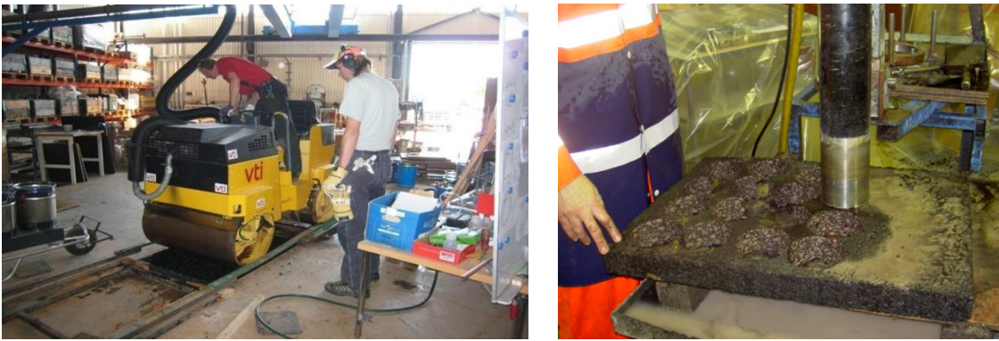
Figure 2: Manufacture of sample slabs
