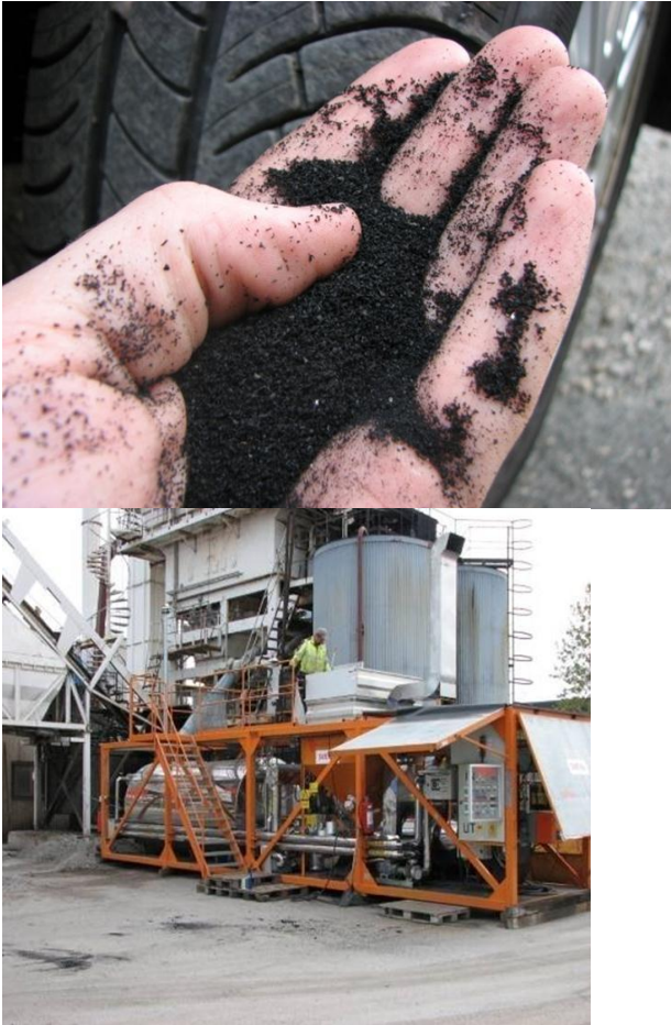
Figure 1: Crumb rubber and rubber blender connected to an Asphalt plant.
