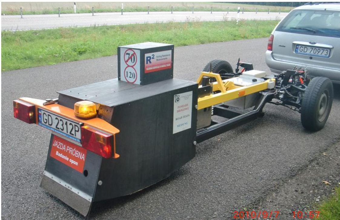
Figure 8: Towed trailer from GUT for measurement of rolling resistance. Photograph courtesy of GUT.
