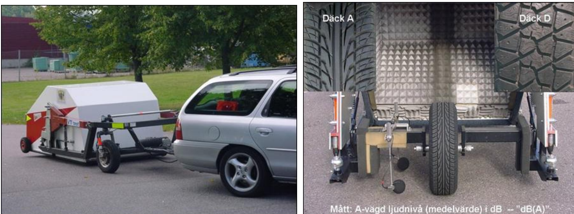
Figure 7: Towed recording device for noise measurement closed (measuring) and open.
