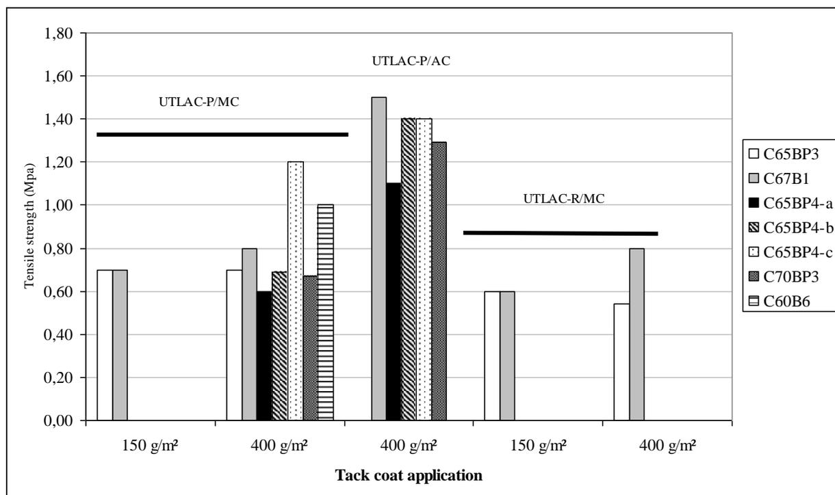
**Figure 7: Shear strength values of ultra-thin surface courses as determined by shear testing**
