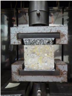
Figure 1: Specimen clamped in the pulling device
