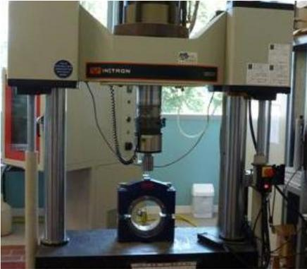
**Figure 3: Shear test device fitted into the testing machine**
