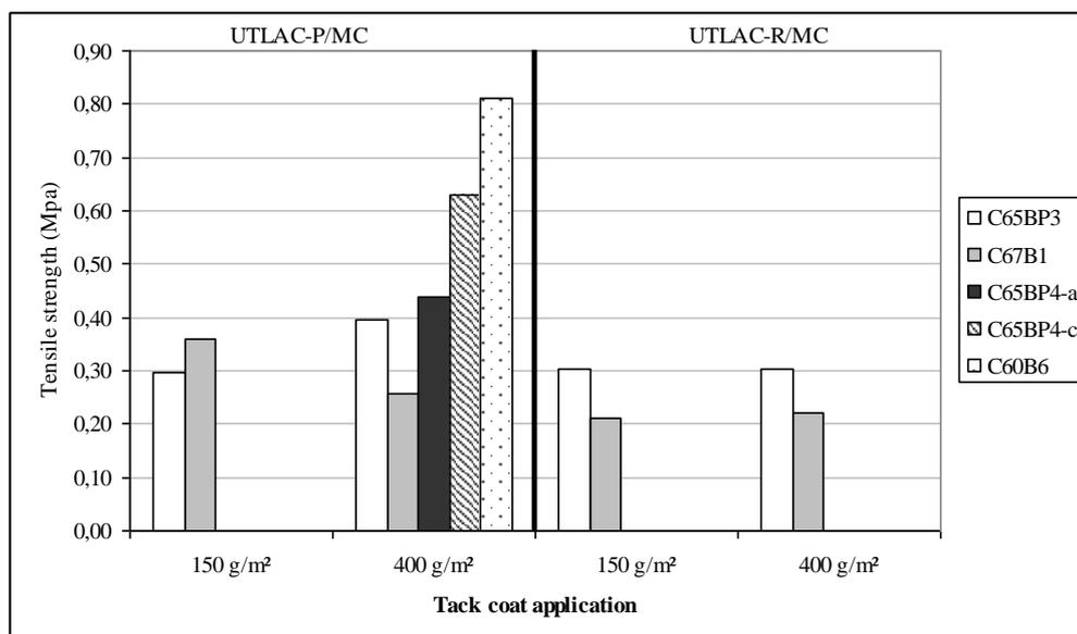
**Figure 6: Strength values for UTLAC layers as determined by direct tensile testing (BRCC method)**
