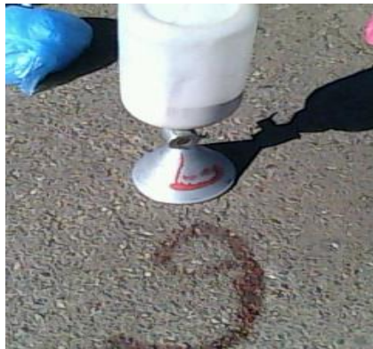
Figure 4: The sand cone apparatus
