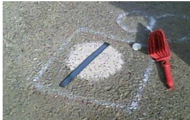
Figure 5: The sand patch method
