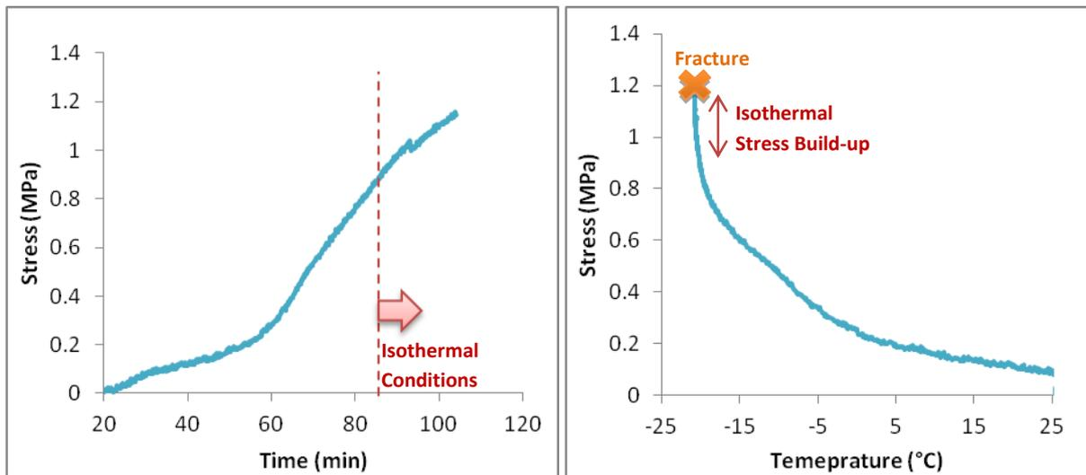
**Figure 7: ATCA restrained beam fracture under isothermal conditions (MN County Road 112-CITGO).**
