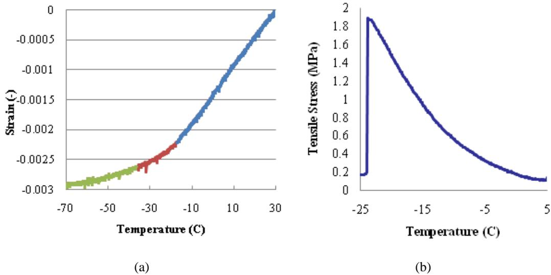
**Figure 2: Typical ATCA result for asphalt (a) Tg (b) stress buildup.**
