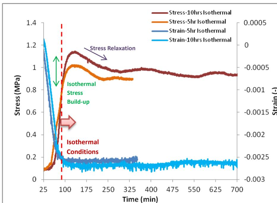
**Figure 3: Isothermal stress behaviour in asphalt after 5 and 10 hrs of isothermal conditions.**
