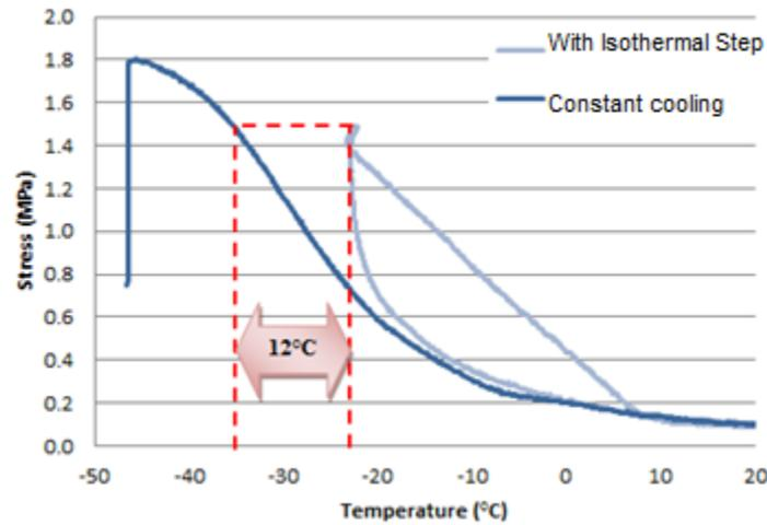
**Figure 5: Typical stress build up in restrained beam using the ATCA, with and without the isothermal conditioning step.**
