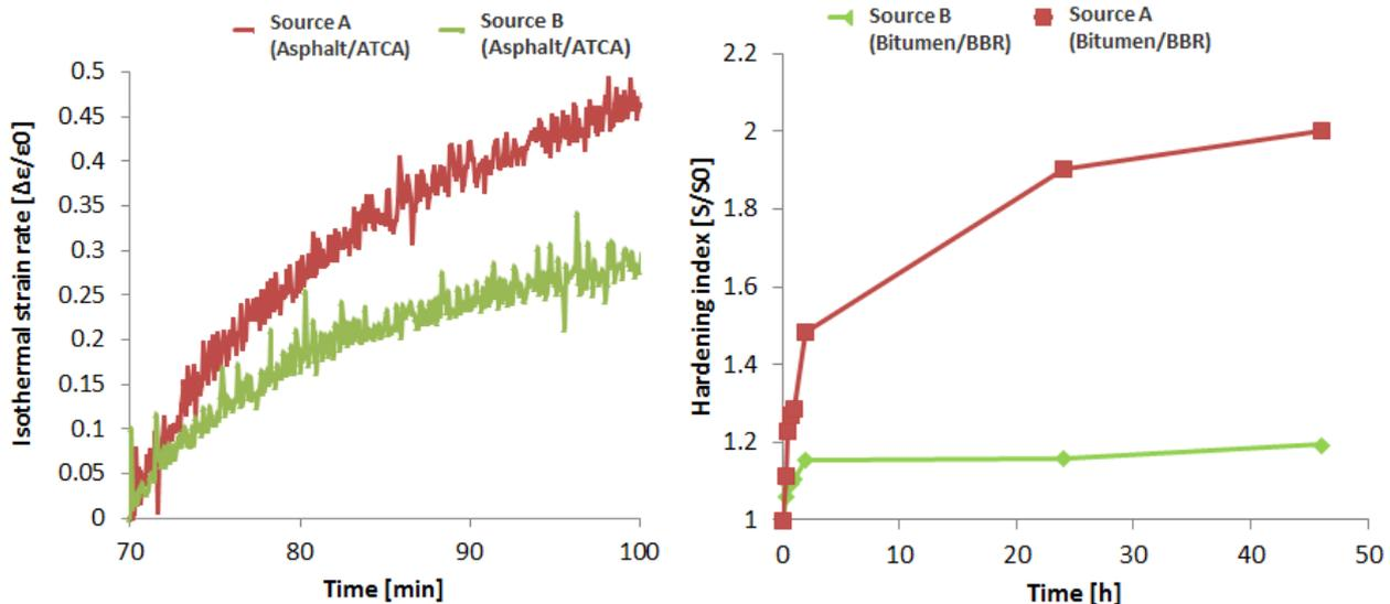
**Figure 8: Comparison of physical hardening susceptibility of two bitumen of identical Superpave performance grades. The field section using asphalt of source “A” cracked two times more than asphalt of source “B”.**
