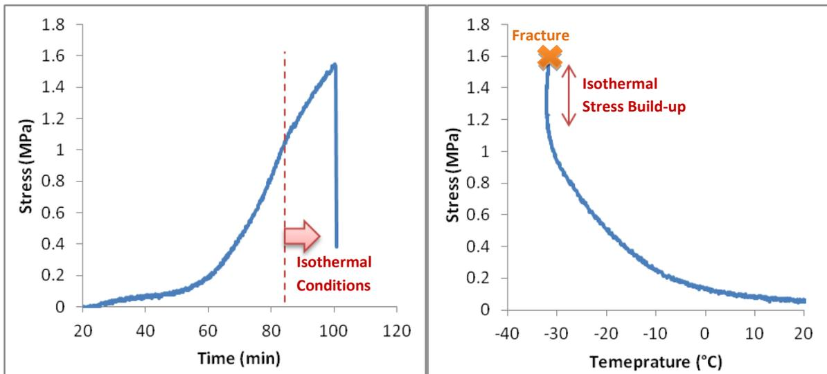
**Figure 6: ATCA restrained beam fracture during isothermal conditions (MN County Road 112-Valero).**
