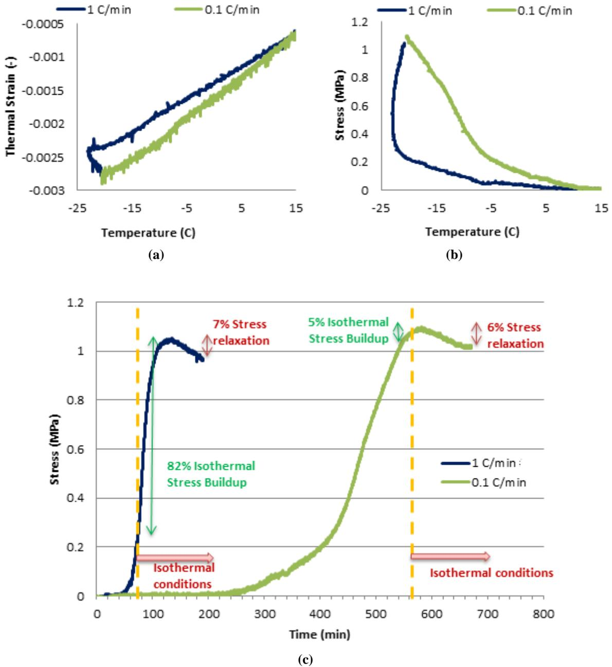
**Figure 4: Comparison of thermal stress and strain during cooling and isothermal conditions at 0.1 and 1°C/min cooling rates.**
